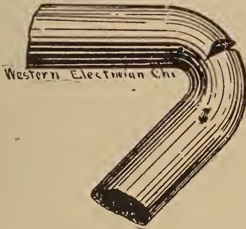
FIG. 32. — SHARP BEND IN A WIRE.
