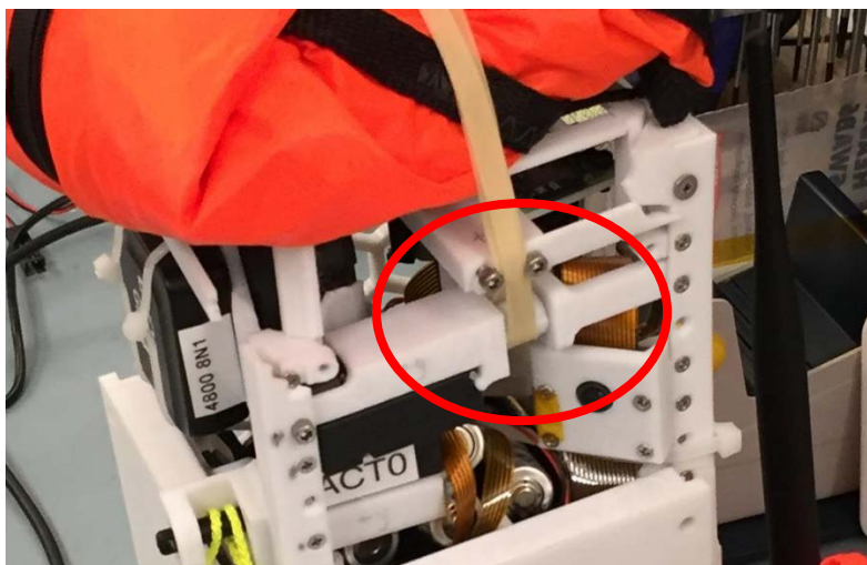
Figure 49. 3D printed sleeve for the actuator axis
