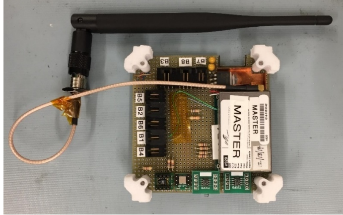
Figure 19. The telemetry antenna and the radio installed on C&DH board
