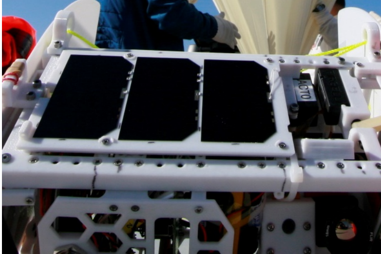
Figure 18. Solar panel on the HAB payload
