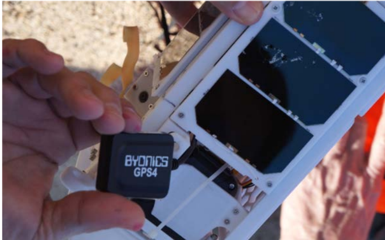
Figure 16. The GPS used on the HAB payload
