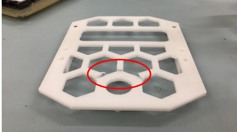
Figure 62. Antenna's face cover damage
