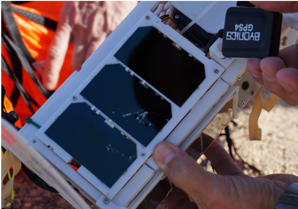
Figure 42. The solar panel damages
