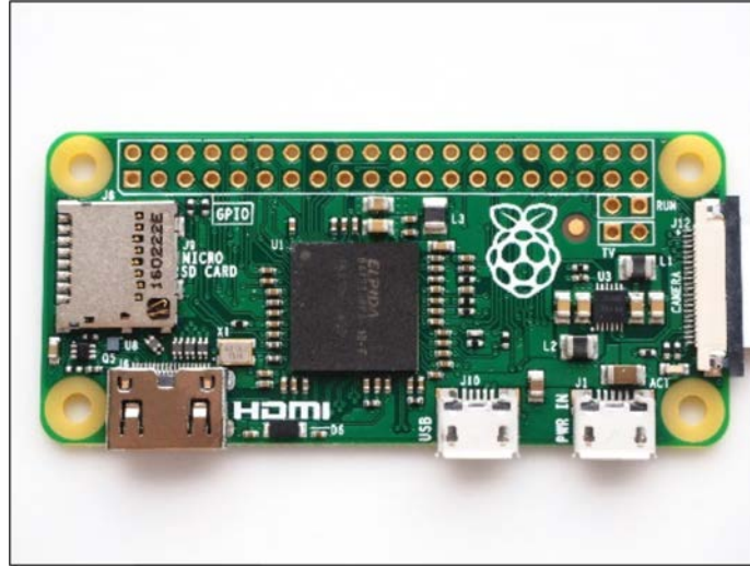
Figure 8. Raspberry Pi Zero board. Source: [12].
