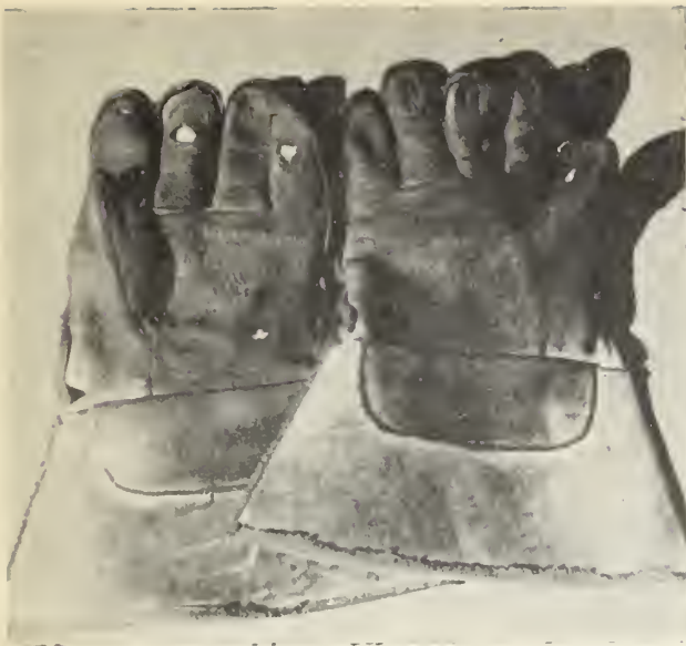
The gloves victim was wearing at the time of the accident. Burns on hand correspond to holes burned in gloves.
