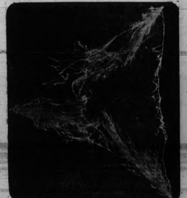
ARTIFICIAL LIGHTNING. —The eye could not catch the exact pattern of artificial lightning flashes recently generated by the General Electric Co. Here is what the camera caught of one. This triangular pattern of lacy light resulted from the discharge of 1,500,000 volts of three-phase alternating current at 60 cycles. The spark points at each corner are nine feet apart.
