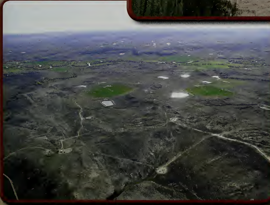
Constructed surface storage ponds and impoundments for CBM-produced water along the Tongue River corridor, south central Montana. Photo courtesy of Jim Bauder, formerly MSU Extension Water Quality Specialist
