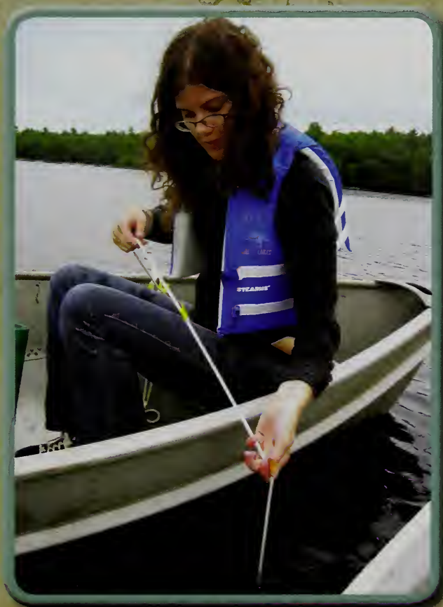
Program volunteers take weekly water clarity measurement using a Secchi disk. These easy-to-perform measurements can be used to assess seasonal and/or long-term trends in lake water clarity and indicate the same trends in water quality and eutrophication.
