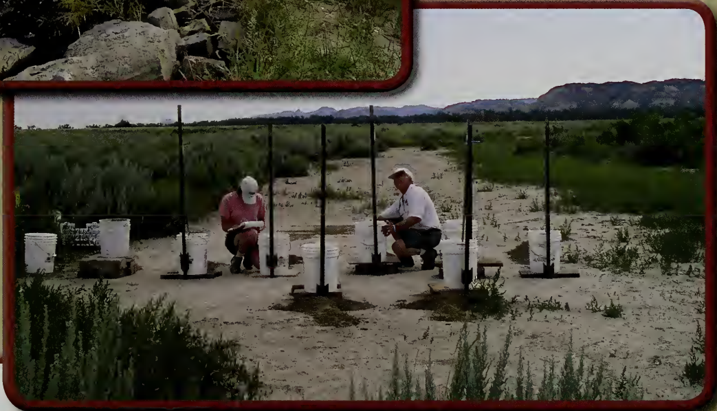
Jim Bauder, former MSU Extension Water Quality Specialist, and Holly Sessoms, former MSU Extension Water Quality Associate, measure infiltration at a CBM water spill site in southeast Montana. Photo courtesy of Suzanna Carrithers, formerly MSU; currently USGS-Bozeman, MT
