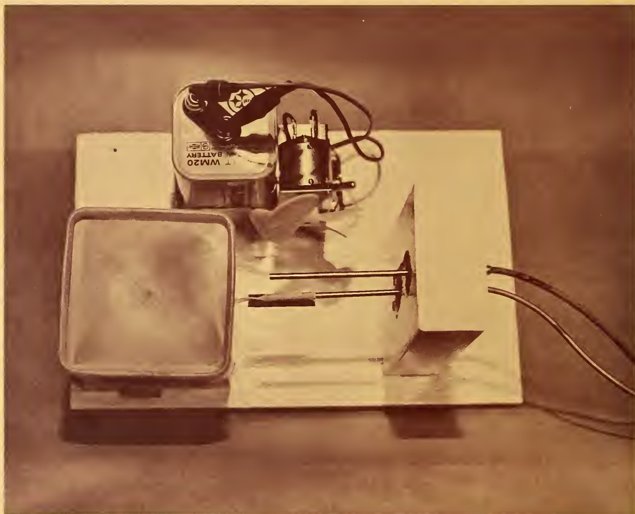
Figure 2.--Thermistor psychrometer used in the recording weather station.
