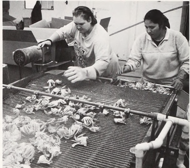
Crab clusters roll out of the cryogenic freezer tunnel where they receive a water glaze to prevent dehydration.
