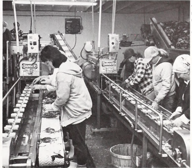
Workers place crabs on an automated backing machine that removes the crabs' backs, viscera and gill feathers.
