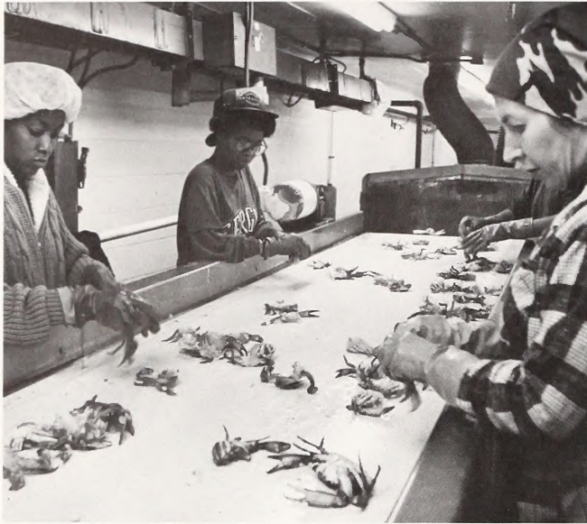
The people in this post-processing inspection line remove improper cuts and miscellaneous pieces prior to cooking.
