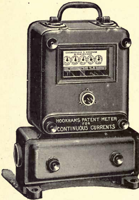
Fig. 288.—Hookham Direct-Current 5000-Amp Meter mounted on Shunt Box
