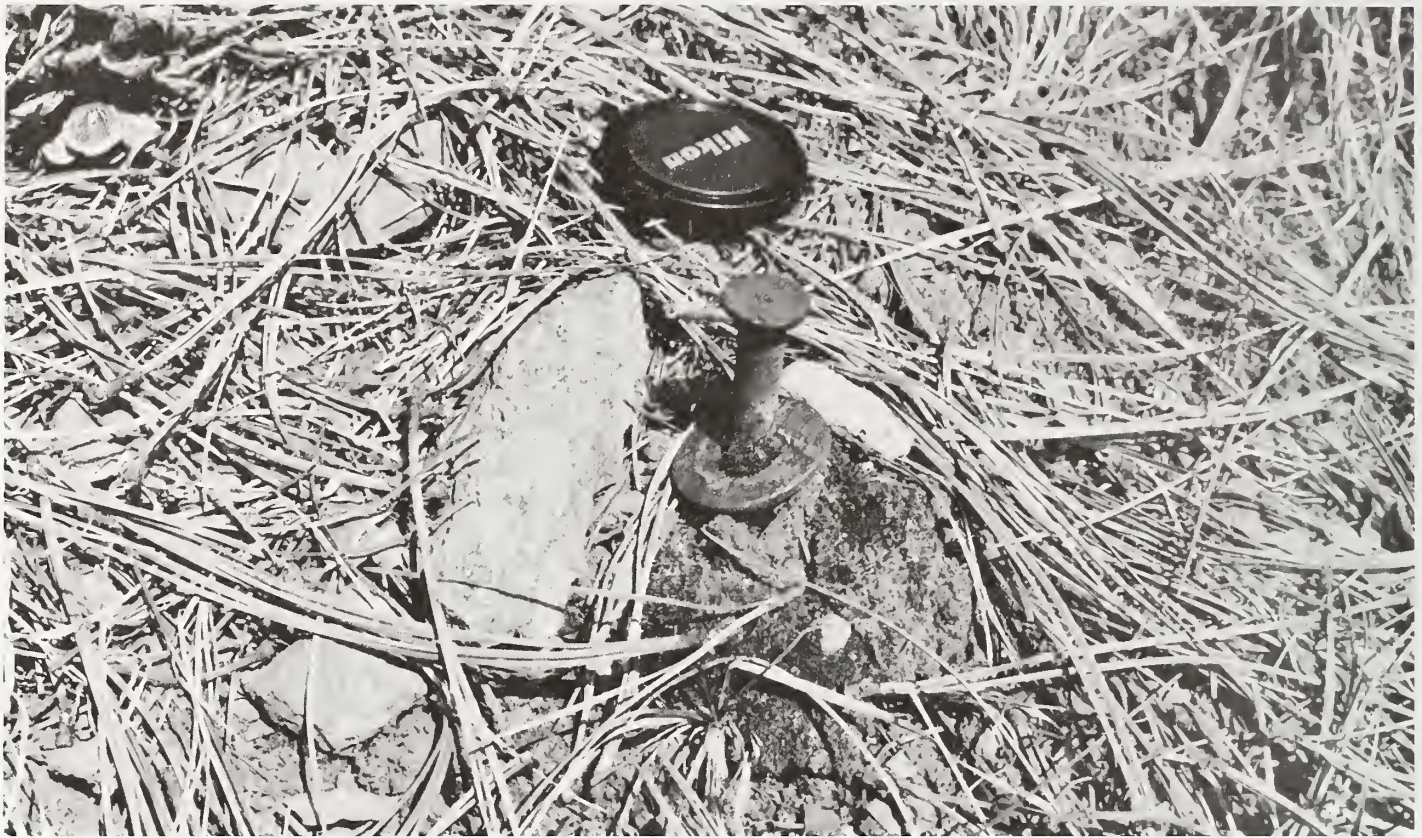
Figure 8. Cryptogamic crust growing through washer, ASLIT, June 1993. The crust incorporates pumice fragments below the washer, and can be seen above the washer, growing through the space between the pin and the washer.
