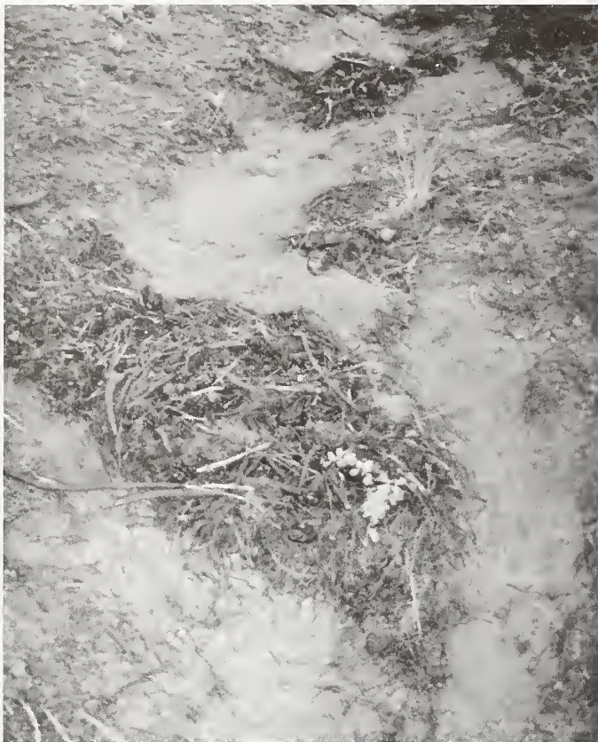
Figure 11. Scoured channel around a plug of organic debris accumulated behind two erosion pins (between rebar stake, left edge of photograph, and the lens cap, lower center), BMMOD, August 1993. The light toned area in the lower half of the photograph is tuff fragments weathering out of the bedrock. The medium toned area is sediment (upper half of the photograph) and scoured soil (lower right half of photograph).
