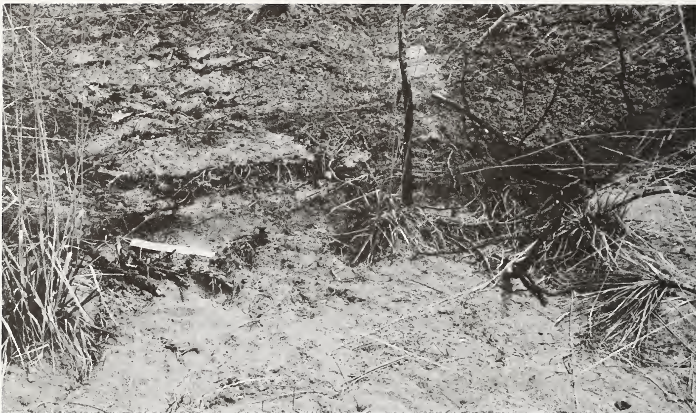
Figure 2. The channel of study basin BMINT in May 1979 where it crosses Transect C (erosion pin #10 in mid-channel, to right of 15cm ruler). Light toned areas are fire-derived deposits of medium to coarse sand-sized quartz crystals and pumice fragments. Medium toned area in upper right of photo results from frost heave disrupting the finer textured ground surface outside of the channel.
