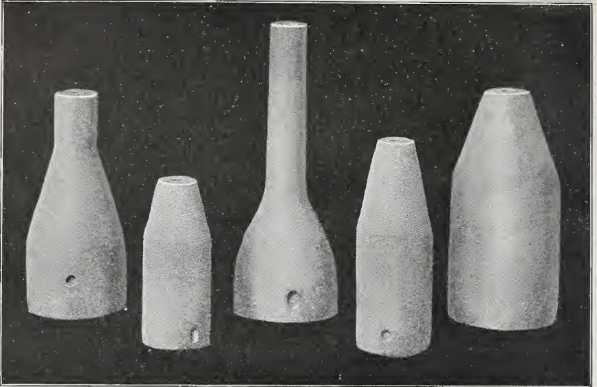
Types of phosphorizers used in the manufacture of phosphor bronze. (Joseph Dixon Crucible Company, Jersey City, N.J.)
