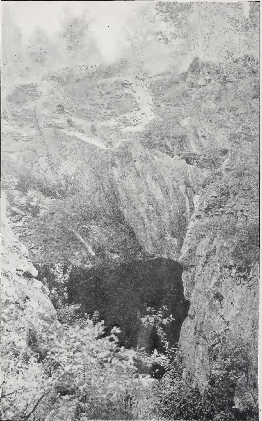
Main pit of Miller mine, range V, lot 10, township of Grenville, Que. The ore-body is stated to have followed the well defined slip face on the far side of the pit.
