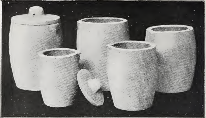
Types of crucibles used in melting non-ferrous metals. (Joseph Dixon Crucible Company, Jersey City, N.J.)
