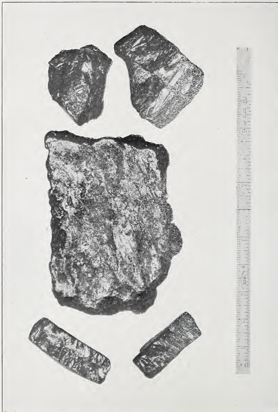
Foliated plumbago, from near Lake harbour, Baffin island. This material is reported to be the equal of Ceylon plumbago for crucible work.
