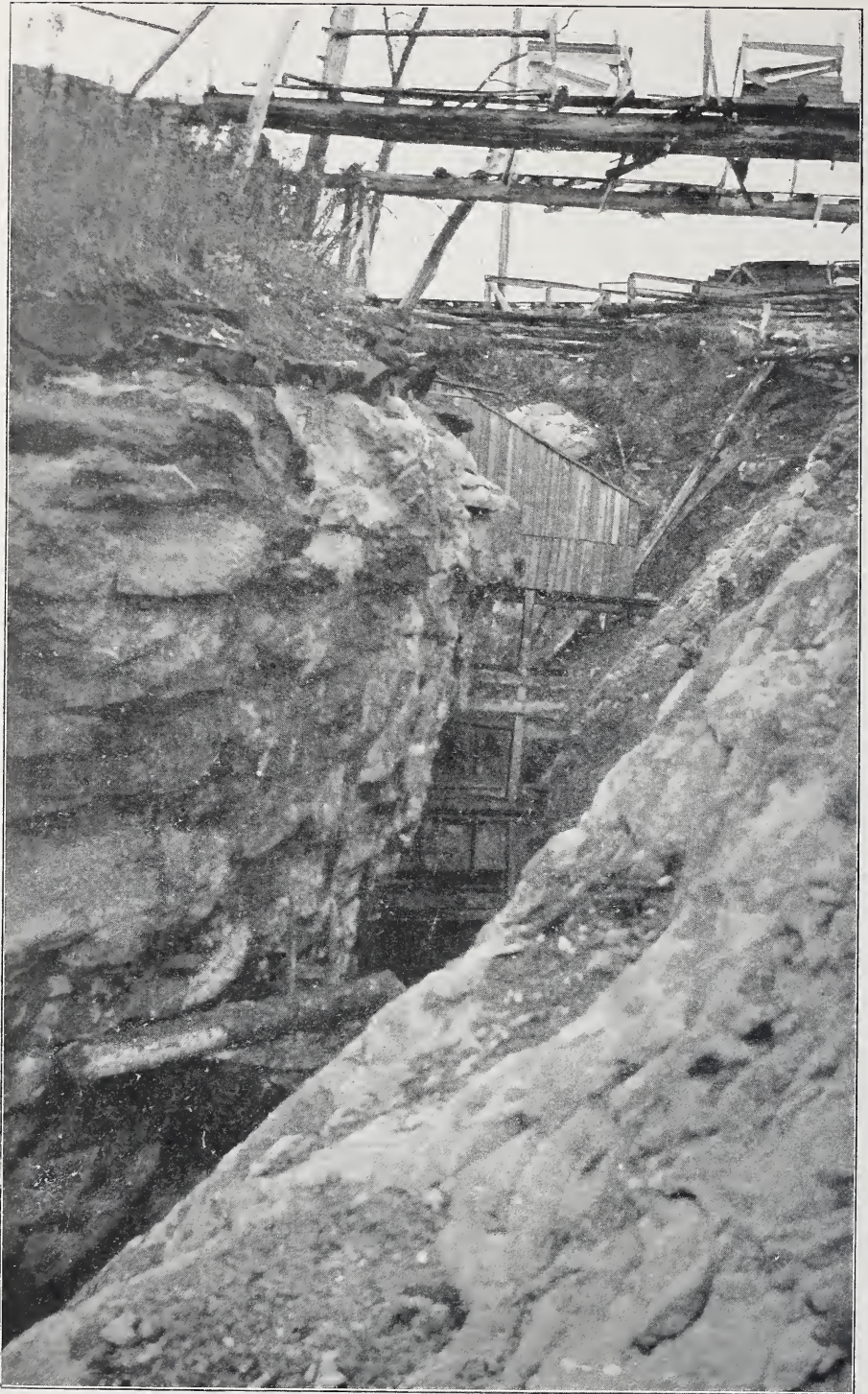
Method of working graphitic limestone ore-body, concession XIII, lot 23, township of Monteaale, Ont.
