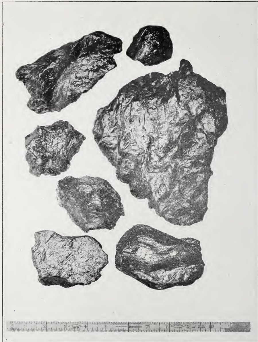
Foliated plumbago, range III, lot 18, township of Low, Que. This plumbago is of good quality, but is hardly as dense as that from Ceylon.
