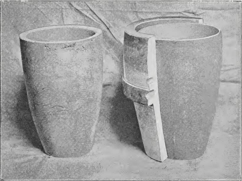
Crucibles as removed from the moulds. (Crossley Machine Company, Trenton, N.J.)
