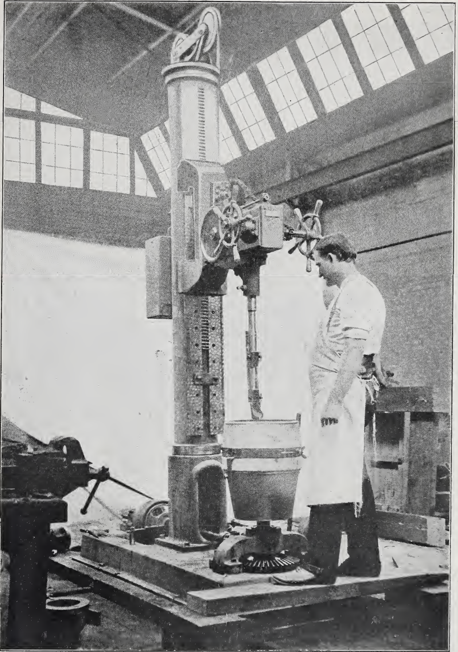
Pull-down and jigger used in making crucibles. (Crossley Machine Company, Trenton, N.J.) The illustration shows the profile or tool in position to be lowered into the mould by means of the right-hand wheel. The left-hand wheel controls the movement of the tool horizontally, in order to press the clay against the wall of the mould.
