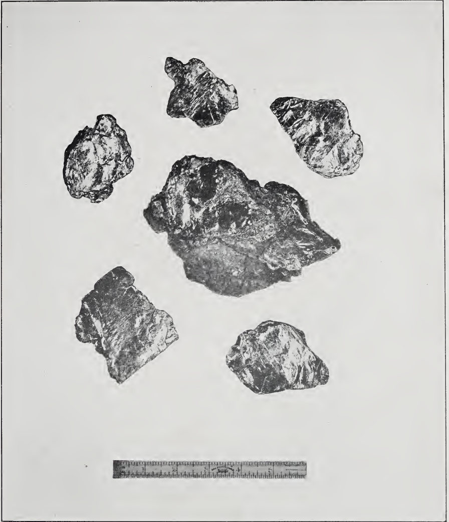
Exceptionally large sized graphite flakes, from range IV, township of Buckingham, Que. The flakes, measuring up to 5 inches across, occur at the contact of a pegmatite dike with gneiss.
