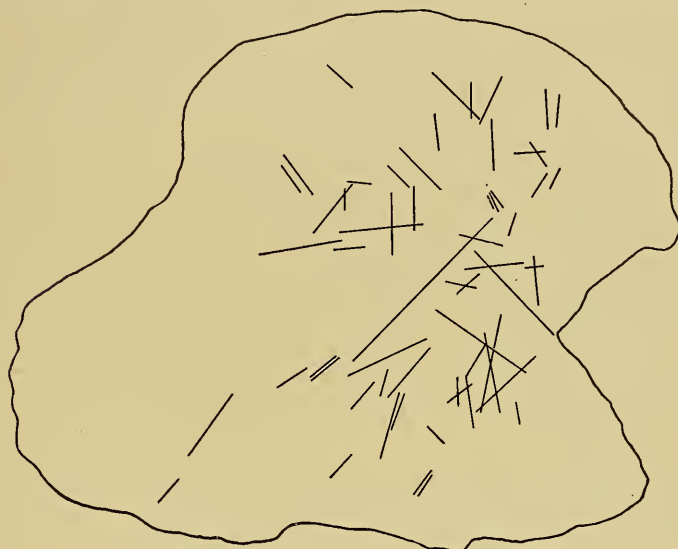
FIG. 10.—Microscopic fractures in granitic quartz.
