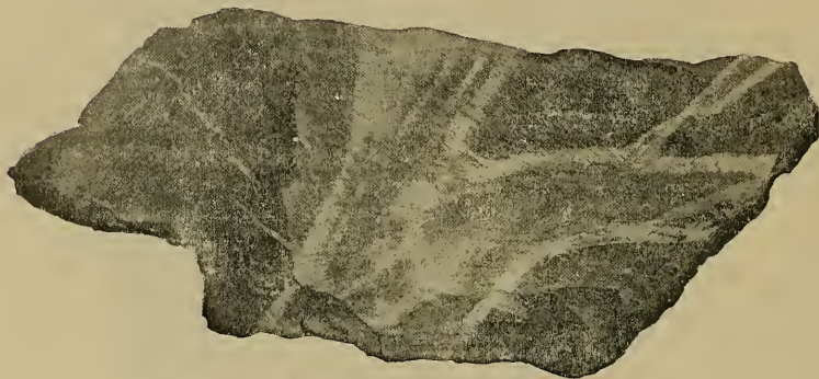
FIG. 2.—Zones of reduction in oxidized fine-grained dolomite.
