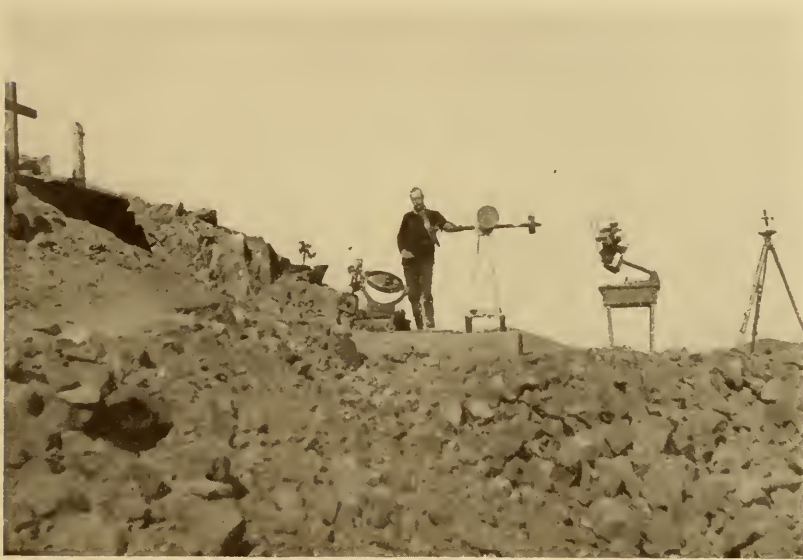
FIG. 33.—Pyranometer, coelostat, pyrheliometers and theodolite with L. H. Abbot, Director at Mount Montezuma.
