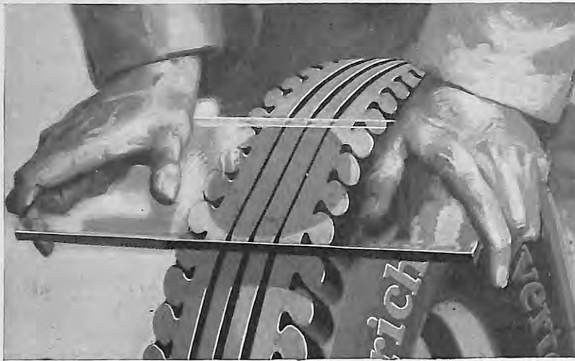
The plate glass test —This glass was pressed against a Goodrich Silvertown till the tread flattened as it would flatten against the road. Note how the center grooves can close up, when the tire is under load.
