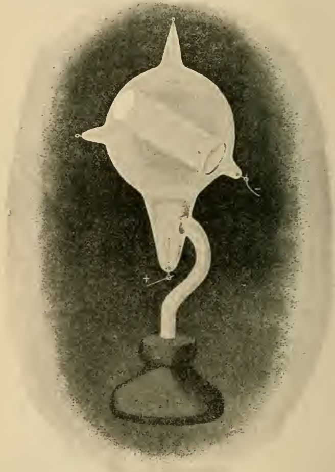
FIG. 2.—A CROOKES' TUBE IN OPERATION.
