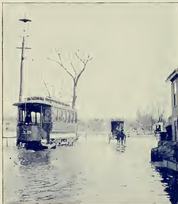
The cars were equipped with G. E.-800 motors and K<sub>2</sub> controllers, and went through the flood without burning so much as a fuse strip.
