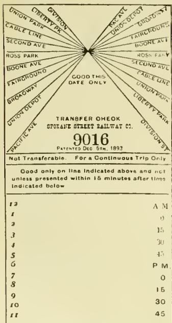
the lower portion of ticket as will leave the hour and minute desired. A small brass strip is used in tearing, thus doing away with the necessity for a punch; or a punch can be used instead if preferred.
