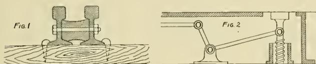
used almost invariably. As shown in Fig. 1, these consist of two ordinary rails bolted together with a filler between. The rails are spiked to ties of oak, a timber which is abundant in Italy.
