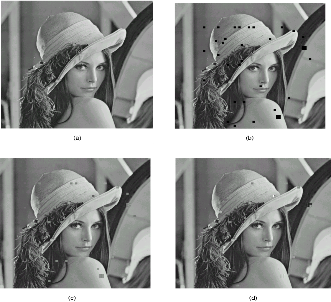
Figure 5.7. (a) Original Image, (b) Image without Error Recovery, (c) Recovered Image Using Linear Prediction, (d) Recovered Image Using Wavelet Based Scheme.
