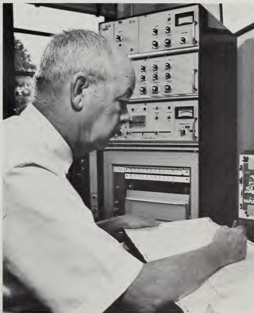
Dr. Underwood examines a profile of maple sap flavor components that was recorded by the gas-liquid chromatograph behind him (1170A1054-11).
