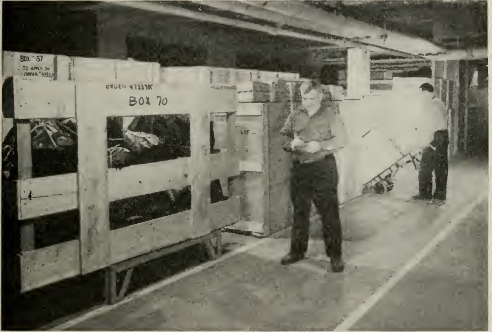
A COMPLETE central office unit, packed for immediate shipment and installation. Comprehensive lists are maintained of the equipment and materials in each of the numbered cases. Box 70, for instance, contains power equipment
