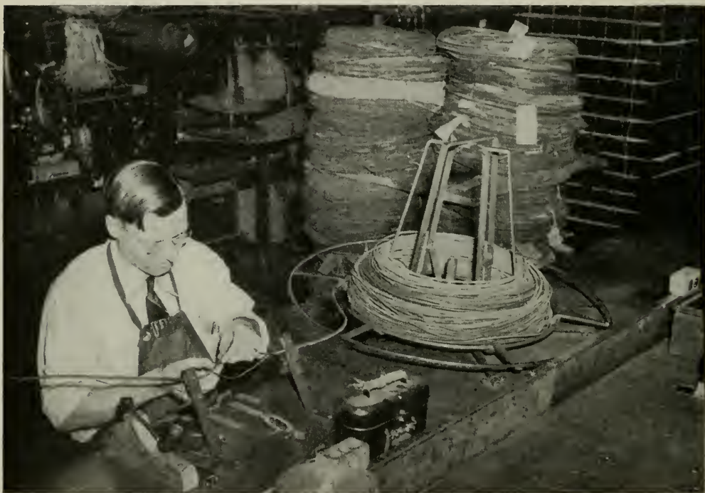
SALVAGED DROP WIRE not in serviceable condition is returned to a Western Electric repair shop, where it is carefully inspected and spliced into convenient lengths
