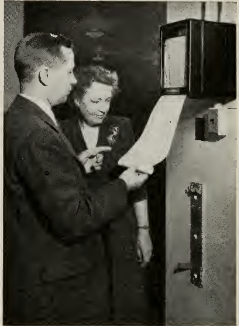
THIS CONTINUOUS RECORD of the volume of stored-up calls is an important aid to the maintenance of satisfactory force adjustment
