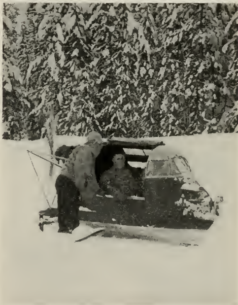
THE SNOWMOBILE: a small, light body mounted on ski runners and driven by an airplane propeller
