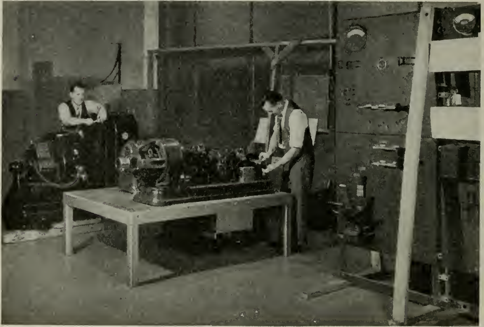
TELEPHONES USE POWER to operate. In this picture, units of power equipment are being reconditioned: left, a battery charging generator; center, a ringing machine; right, a power distribution panel
