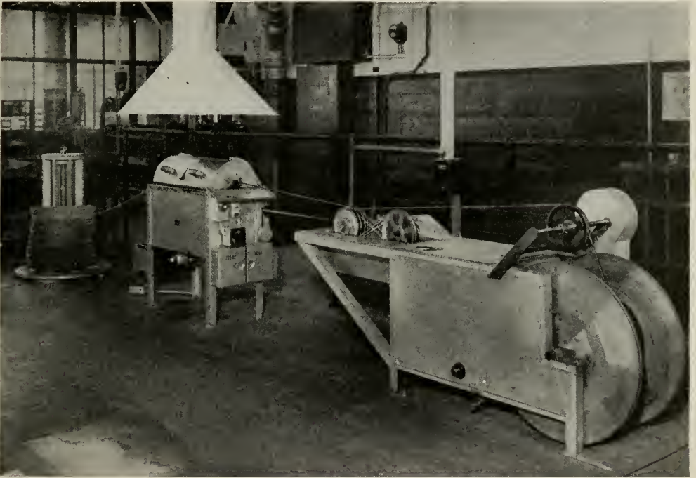
SPECIALLY DESIGNED APPARATUS is used to re-impregnate drop wire with weather-proofing compound. Left to right: pay-out reel, compound tank, setting tank, and take-up reel
