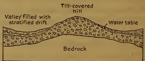
FIGURE 10.—Diagram showing the relation of the water table on hills to the water table in valleys in glaciated regions.
