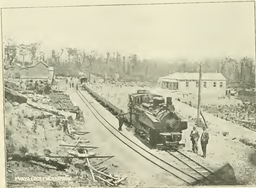
HAGAN'S PATENT 40-TON 2-FOOT GAUGE ENGINE AND TRAIN.
