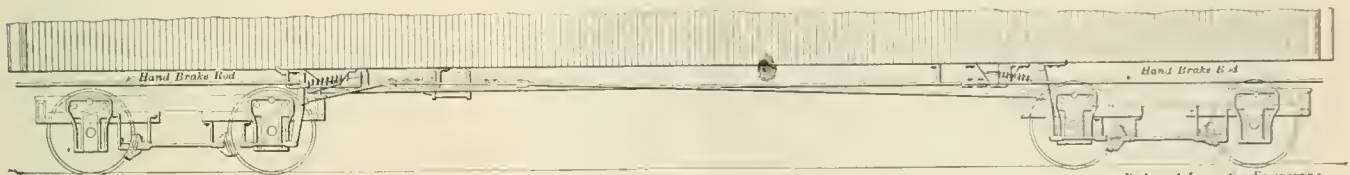
SHELTON BEAMLESS BRAKE AS APPLIED TO DENVER & RIO GRANDE R. R. COACH No. 703.
