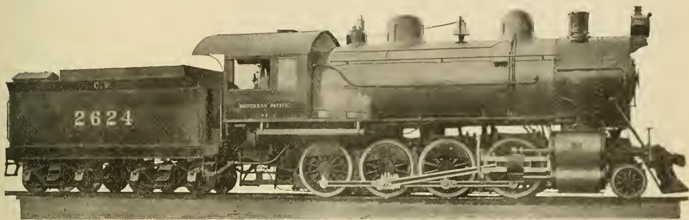
IDEAL FREIGHT ENGINE BUILT BY BALDWIN LOCOMOTIVE WORKS. CYLINDERS, 17 AND 28x30 INCHES; DRIVERS, 57 INCHES DIAMETER; WEIGHT, 204,800 POUNDS; HEATING SURFACE, 3,600 SQUARE FEET; TRACTIVE POWER, 40,000 POUNDS. CAN HAUL 1,500 TONS UP GRADE, 50 FEET TO THE MILE.
