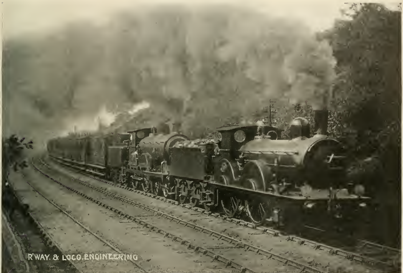
THE CROMER EXPRESS—GREAT EASTERN RAILWAY. THIS IS THE SHOW TRAIN ON THE "POOR MAN'S LINE"—131 MILE RUN IN 2 HOURS 38 MINUTES. AVERAGE SPEED, 49.7 MILES PER HOUR WITH HEAVY TRAIN. PHOTOGRAPH TAKEN WHEN ASCENDING BRENTWOOD BANK, A GRADE OF 1 IN 100.
