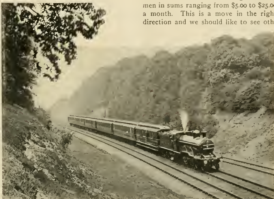
GREAT NORTHERN OF ENGLAND—ATLANTIC TYPE ENGINE, VESTIBULE CORRIDOR CAR TRAIN, LONDON-LEEDS SERVICE. PULLMAN VESTIBULES WITH GOULD AUTOMATIC COUPLERS THROUGHOUT.
