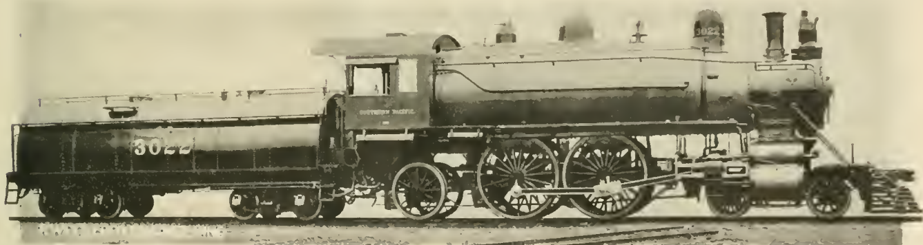
ATLANTIC TYPE, OIL BURNING COMPOUND FOR THE SOUTHERN PACIFIC.
