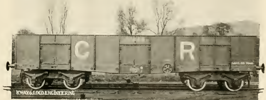
CALEDONIAN NEW 30-TON BOGIE WAGON.
