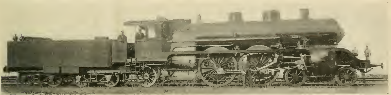
GERMAN FOUR-CYLINDER ATLANTIC TYPE COMPOUND.
