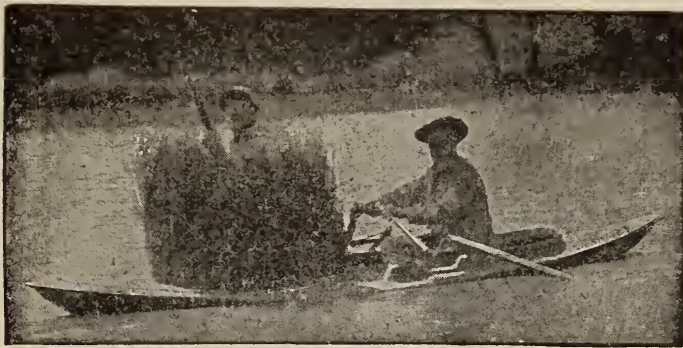
"GET THERE" SAFETY DUCKING BOAT, WITH GRASS BLINDS AND BOW FACING OARS
