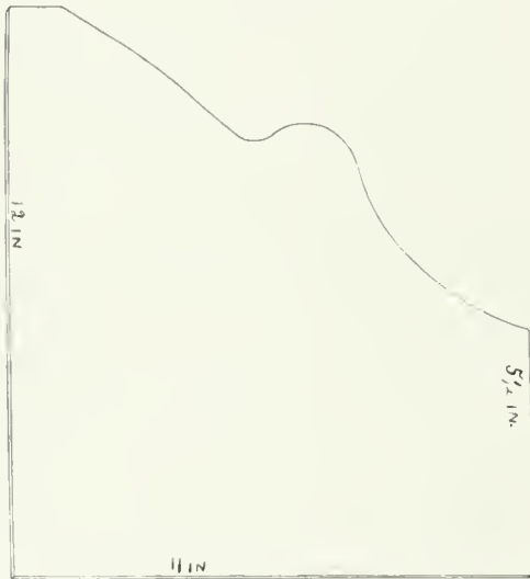
FIG. 5. Lead-rubber shield for side of face, ear, side of neck and shoulder.
