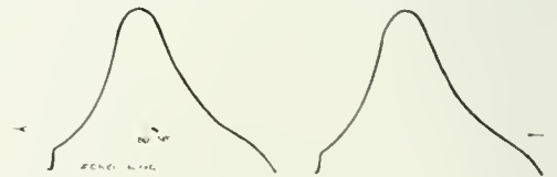
FIGURE 4 FOUR ARM RECTIFIER IN CLOSE ADJUSTMENT WITH RHEOSTAT CONTROL
