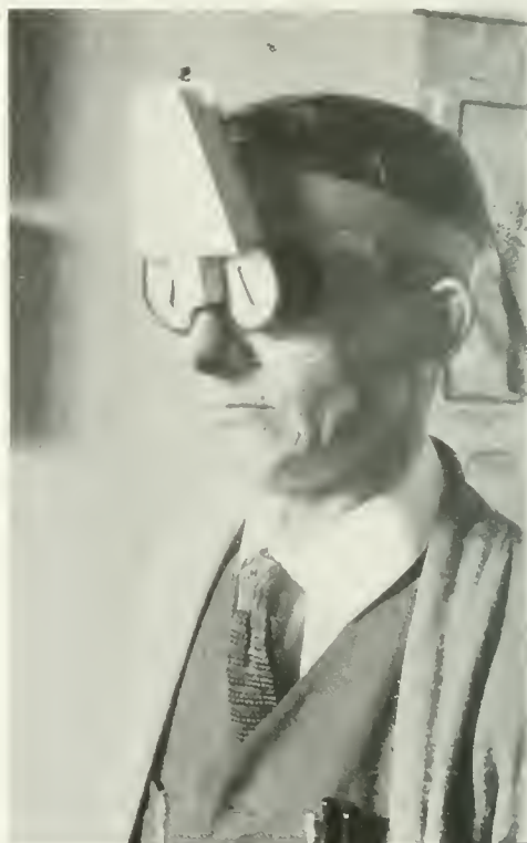
FIG. 5. The shutter can be pushed away from in front of the eyes without removing the strap.
