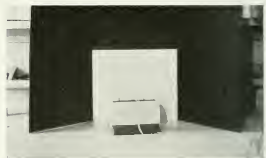
Solid lead block for housing radium needles, eye only protruding for threading.
