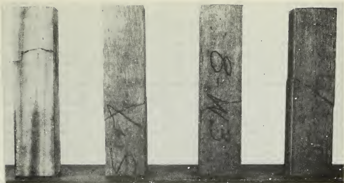
Fig. 7.-Angular shearing failures in compression parallel to grain tests for green tabonuco.
