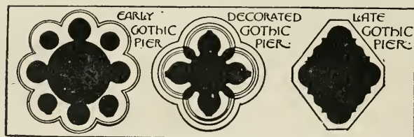
GOTHIC FORMS FROM WHICH THE TREFOIL AND QUATREFOIL DETAILS WERE TAKEN, OBTAINED BY THE USE OF CIRCLES
