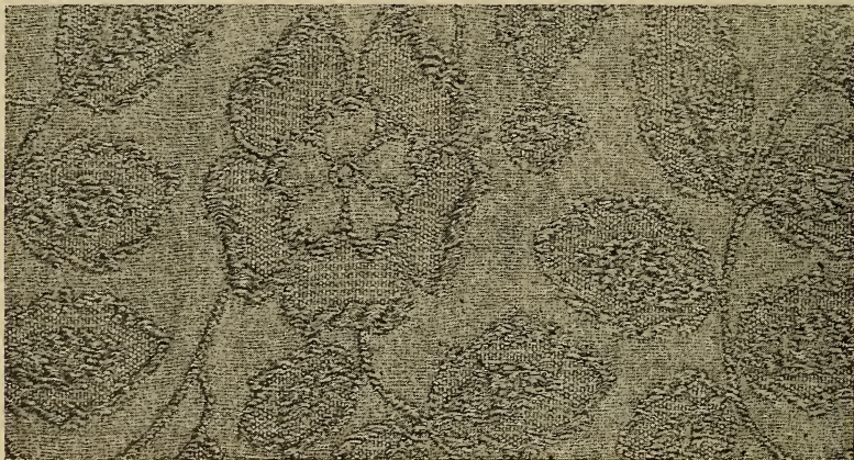
A Novelty Fabric of Unusual Interest Showing Jacquard Weave on Crepe Cloth.
