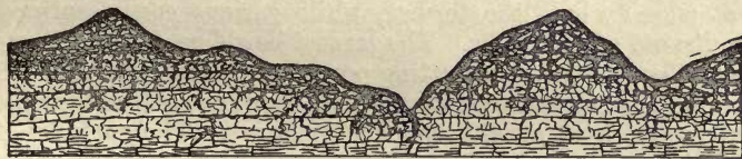
FIG. 17. Diagram showing the relation of mantle rock to the underlying rock from which it was derived. (Courtesy of U. S. Geol. Surv.)
