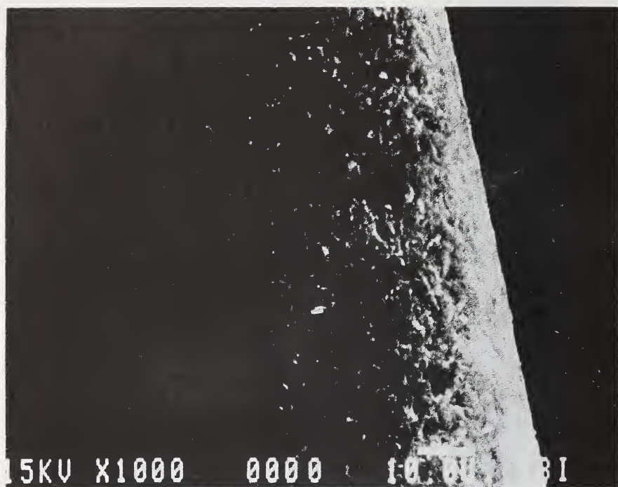
FIGURE 6. Hair after 30 minutes of treatment with sodium hydroxide
