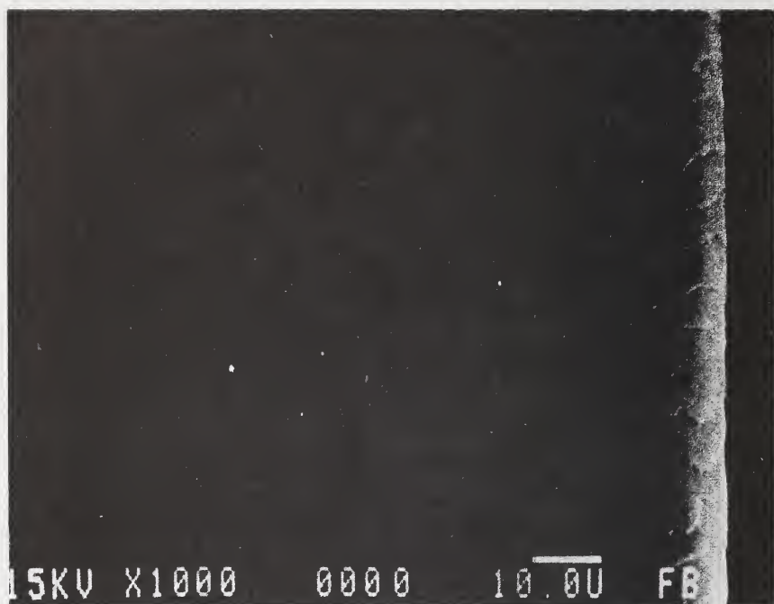
FIGURE 10. Hair after 30 minutes treatment with hydrochloric acid
