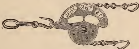
Fig. 8.— Pulley in Messrs. Davey, Sleep, and Co.'s Three-horse Whippetree , No. 413.
