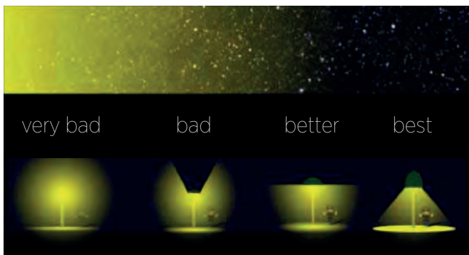
Figure 3. Outdoor Lighting Codes regulate not only the brightness, but also the directionality of light. Unshielded lights shine indiscriminately in all directions, polluting the sky and wasting energy. Shielded fixtures direct light where it is needed. © Canadian Space Agency.
