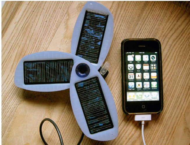
Figure 3.3 Solio hybrid charger powering mobile phone. Image compliments Alan Levine, public domain.
