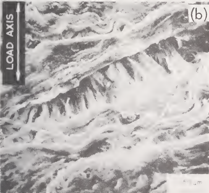
FIGURE 5. Dermal collagen under load (After Millington et al., in Kenedi, [11]). (a) "Scissor" action. (b) Transverse splitting.
