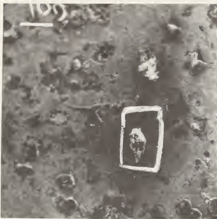
FIGURE 6. Scanning electronmicrograph of porous palladium electrode; magnification 100; 97 percent palladium 3 percent PMMA; sintered at 450 °C.
