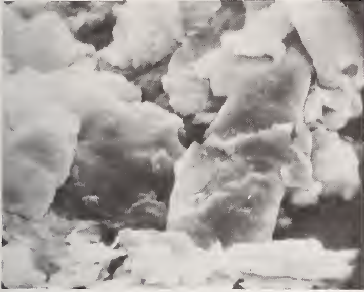
FIGURE 9. Stainless steel 316L ball milled for 192 hours in a rotary ball mill.
