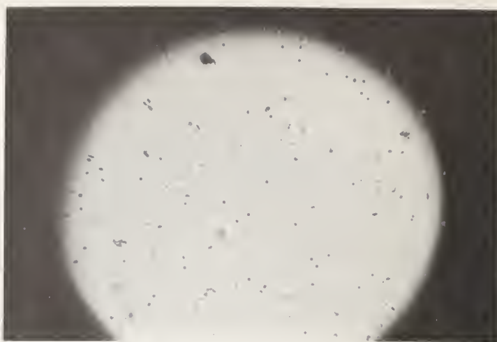
FIGURE 2. Low power ( \times 40 ) photomicrograph of HEP-2 cell growth on a poly-TFE coated cover slip. This represents a 4+ toxic reaction.
