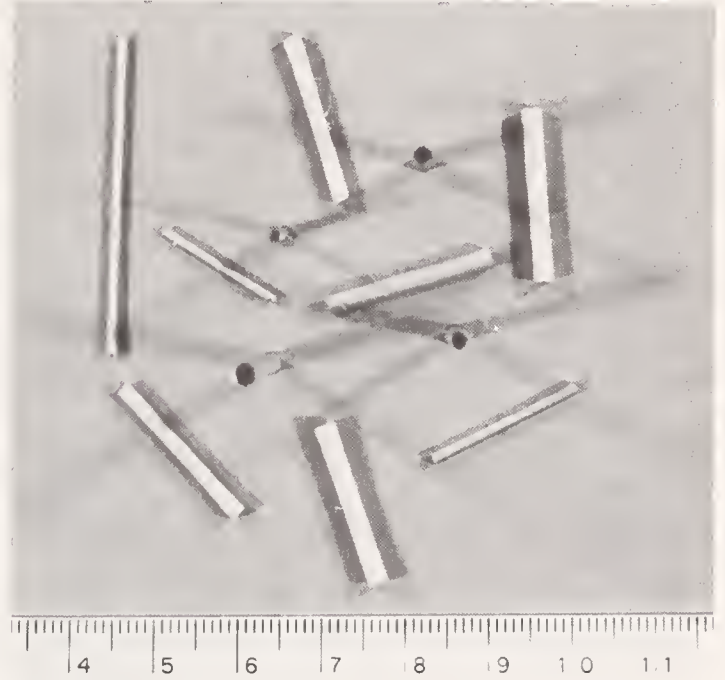
FIGURE 11. Various porous tubes made by slurry coating-sintering process.
