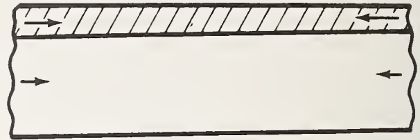
FIGURE 3. Development of interfacial stresses between a flame spray coating and a prosthesis due to thermal expansion mismatch.
