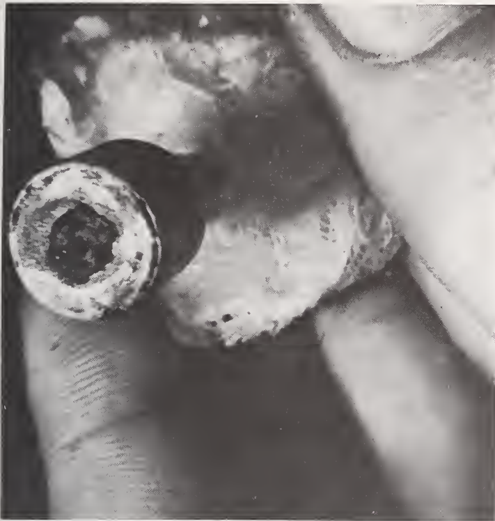
FIGURE 29. Fractured end of the flame spray coated segmental implant showing the exposed metal surface fracture site (grey areas).
