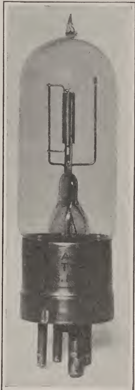
The WD-11 tube, which operates on a single dry battery cell.
