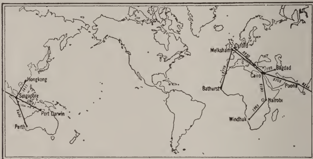
British Imperial scheme of 1919 for radio communication. This is a less ambitious but more practical scheme than that of 1913. London is connected with distant points by means of short spans and relays, so that the distances are entirely feasible.
