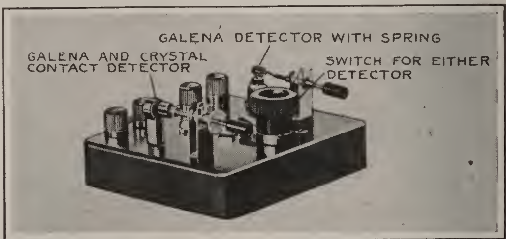
A crystal detector unit. In this case two detectors are mounted on the same base, with a switch for selecting either detector.
