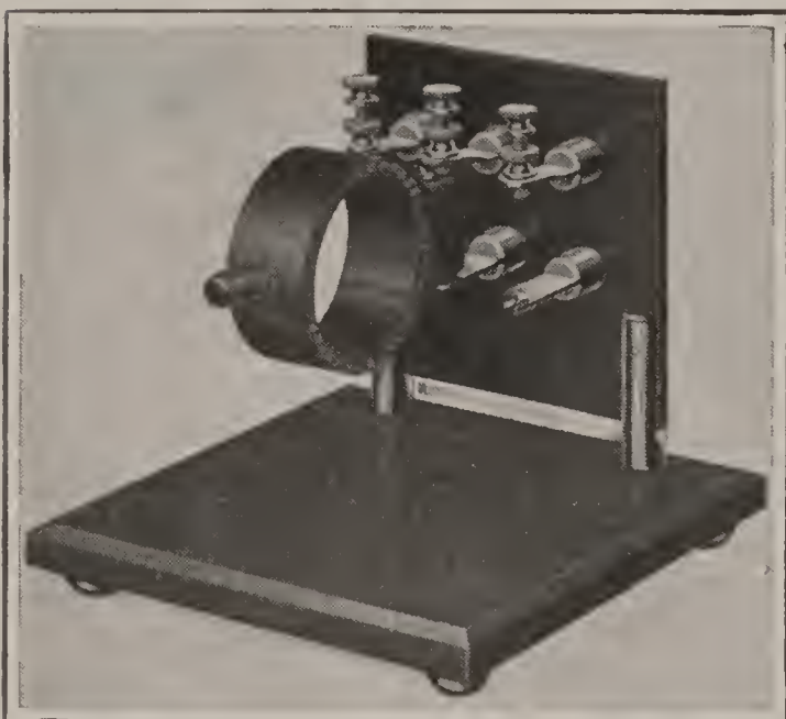
One style of mounting which takes two or three compact inductance coils for a loose-coupler, and tickler coil combination when using a regenerative circuit.
