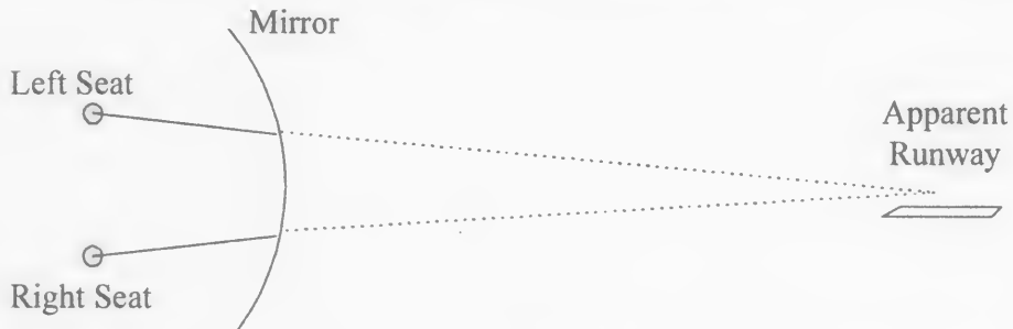
Figure C2J - Runway view in a collimated display
