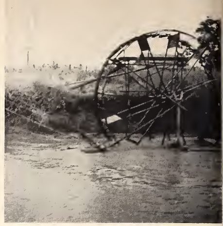
Floating water wheel elevates river water for irrigation of small fields.
