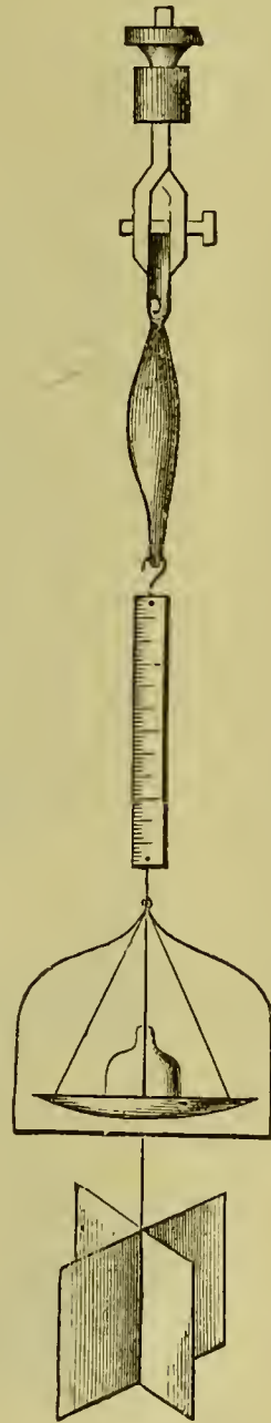
FIG. 7. DU BOIS-REYMOND'S APPARATUS FOR THE STUDY OF ELASTIC EXTENSION IN MUSCLE.
