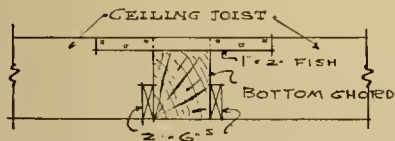
DETAIL SHOWING HOW CEILING JOISTS ARE SUPPORTED ONTO BOTTOM CHORD OF TRUSS
