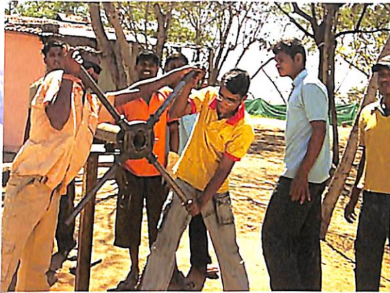
Community service - students doing threading of pipe
