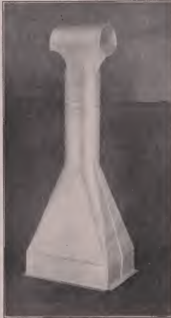
Problems 107 and 108. Base for Chimney Top and Hood.
