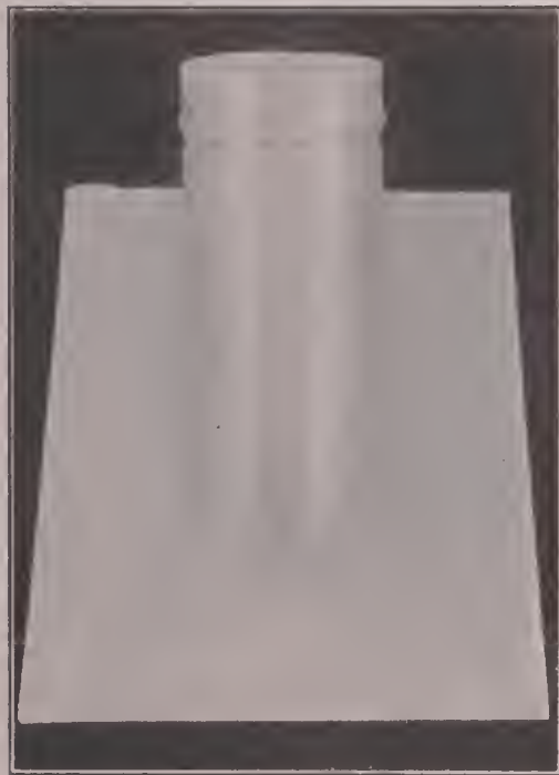
Problem 5. Pipe and Roof Flange.
