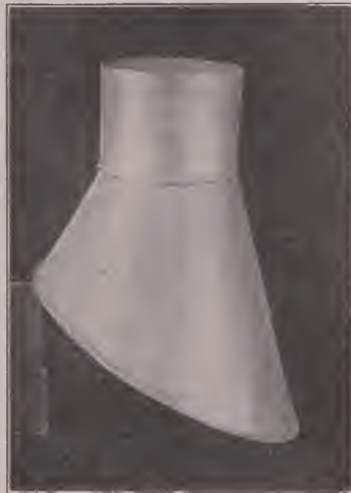
Problem 80. Irregular Flaring Roof Collar.
