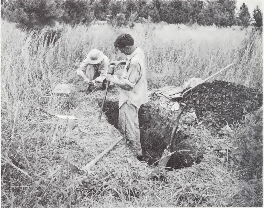
Figure 14.—Collecting samples in an old field just beginning to seed in naturally to pine. From the samples it is possible to determine the percolation rate, pore-size distribution, and bulk density of the soil. The man in the pit is operating a soil-sampling apparatus.
