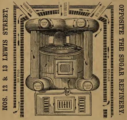
This is the name of a Furnace constructed on an entire new principle, for the purpose of warming dwelling houses, public buildings, halls, hospitals, &c., &c. It differs essentially from other Furnaces, by having an immense radiating surface, and a creative draft.
