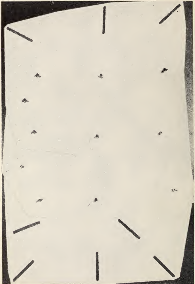
FIGURE 8.—Slotted templets. The shafts of the studs are pierced, as shown, so that the position of the center of the stud can accurately be recovered.
