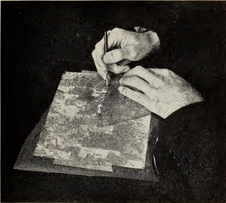
FIGURE 7.—Drawing the radials on a transparent hand templet.
