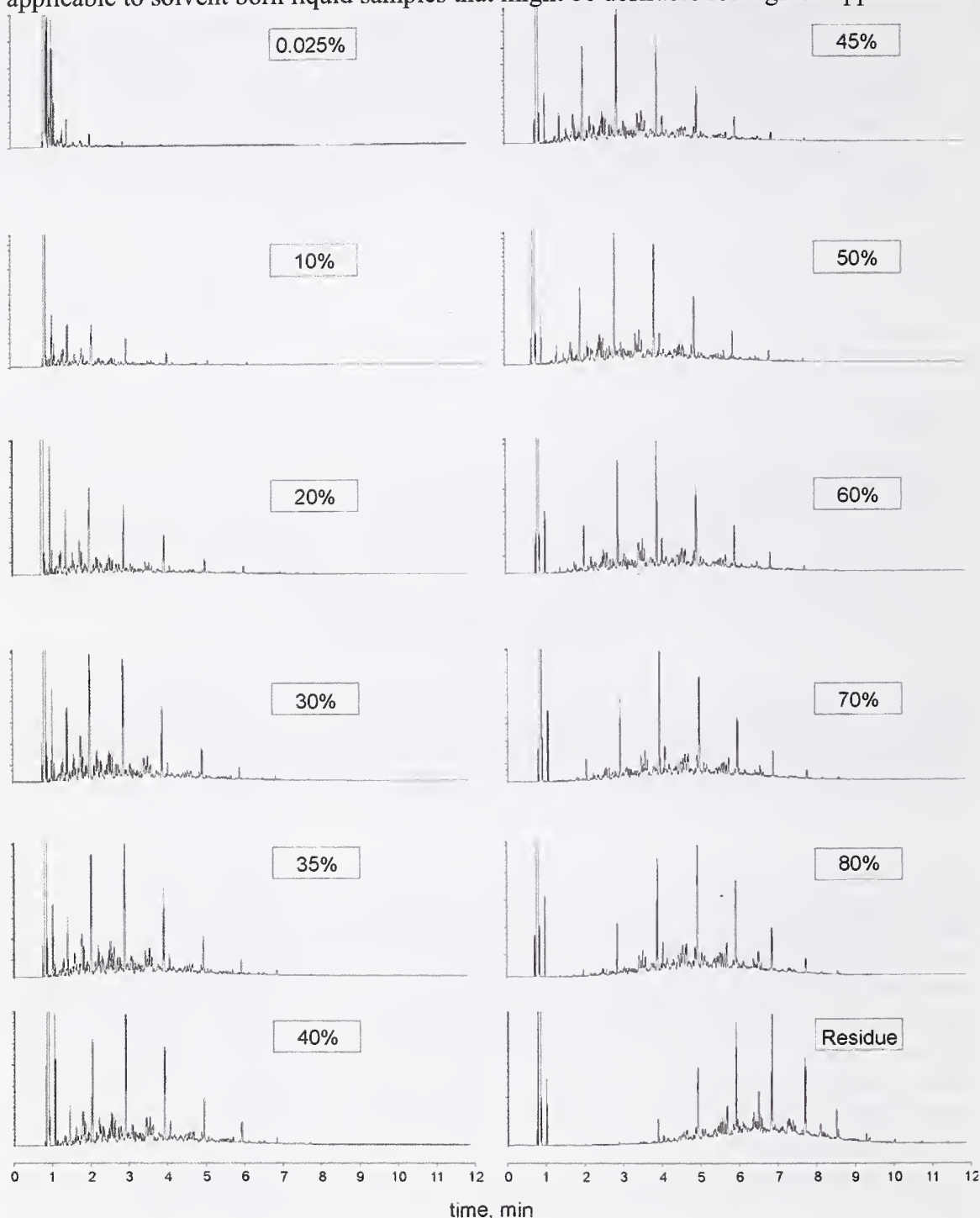
Figure 24: Chromatograms of distillate fractions of a typical Jet-A sample, in this case Jet-A-4658, presented in arbitrary units of intensity (from a flame ionization detector) plotted against time. One can see the solvent peaks very early in the chromatograms. The details of the chromatography are discussed in the text.
