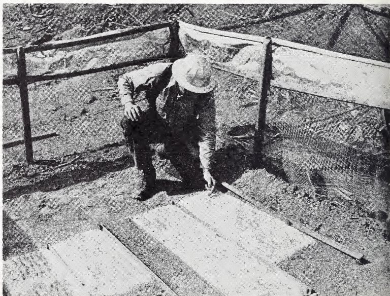
Artificial seedbed study was made to explore ways of overcoming seedling losses due to hot seedbed conditions. Seedbeds shown above were white silica sand of different size particles. Other seedbed materials included basalt gravel, mineral soil, needle litter, vermiculite, and charred surface material.
