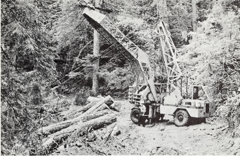
The mobile yarder-loader machine used for salvage logging in old-growth residual stands.
