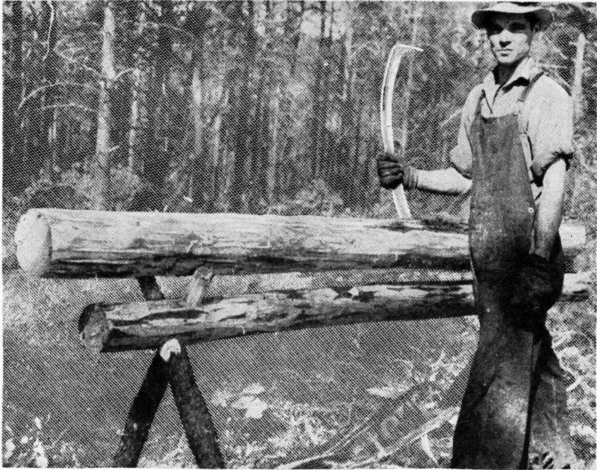
FIGURE 14.—Bench for holding bolt during peeling.
