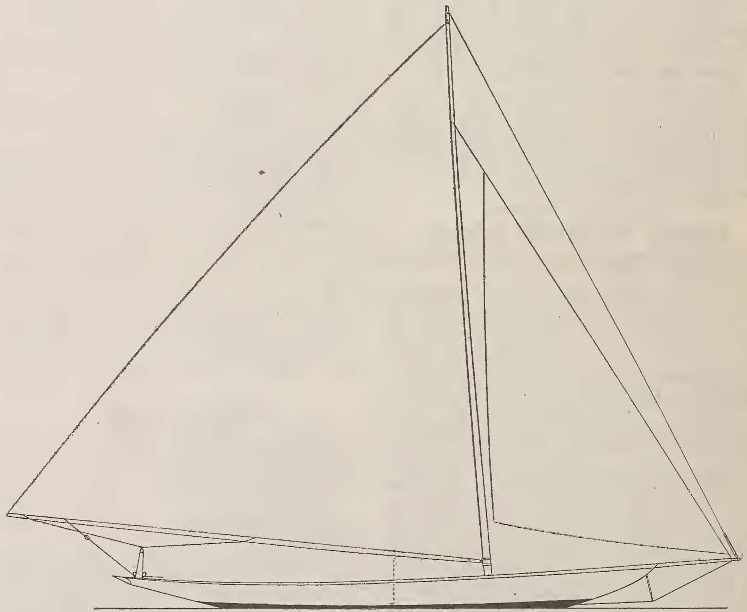
21-FOOT BERMUDA SLOOP—SAIL PLAN. Designed by Fred. M. Hoyt. Built by the Greenport Basin & Construction Co.
