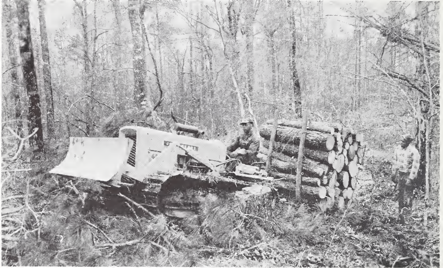
Figure 26 — Tractor roads in moderately steep country often require little preparation. (Courtesy Deere and Company)
