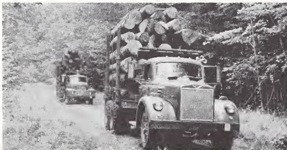
Figure 22 — Tandem-axle trucks of a 30,000 to 35,000 lb. Gross Vehicle Weight size are a common log-hauling vehicle in the Northeast. They carry upward of 2,000 bd. ft. of logs and require well-constructed woods roads.
