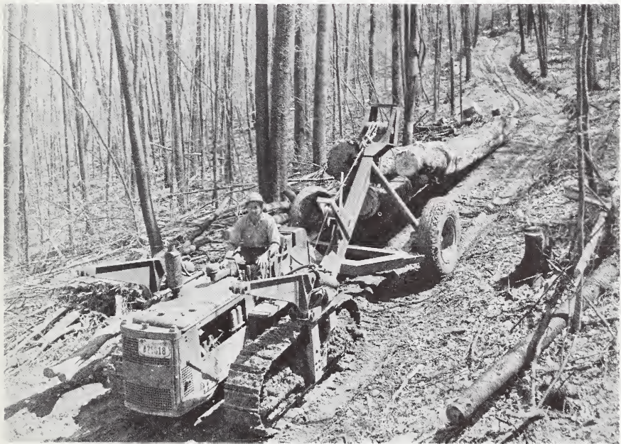
Figure 29 — Tree-length skidding with tractor and arch requires carefully located roads. Alignment of road is important.
