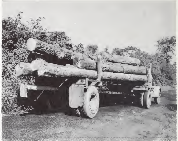
Figure 23 — The tractor-trailer type of log truck makes for economic transportation but its use requires well-engineered roads.
