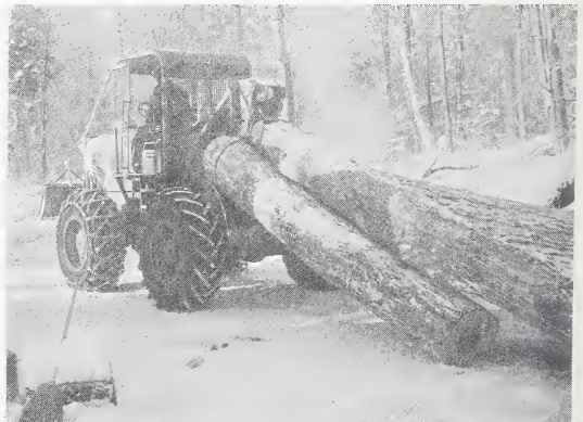
Figure 27 — Fast four-wheel power skidders such as this are well suited for tree-length skidding over long distances. They perform under many adverse conditions but operate most efficiently on well-located roads.
