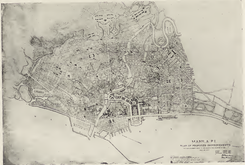
PLAN FOR THE DEVELOPMENT OF MANILA, SUBMITTED TO THE PHILIPPINE COMMISSION BY D. H. BURNHAM AND PEIRCE ANDERSON IN 1905. THE ESSENTIAL ELEMENTS ARE THE GOVERNMENT CENTER AND PROPOSED ARTERIES RADIATING FROM IT, THE RAILWAY STATION AND THE SHORE ROAD.
