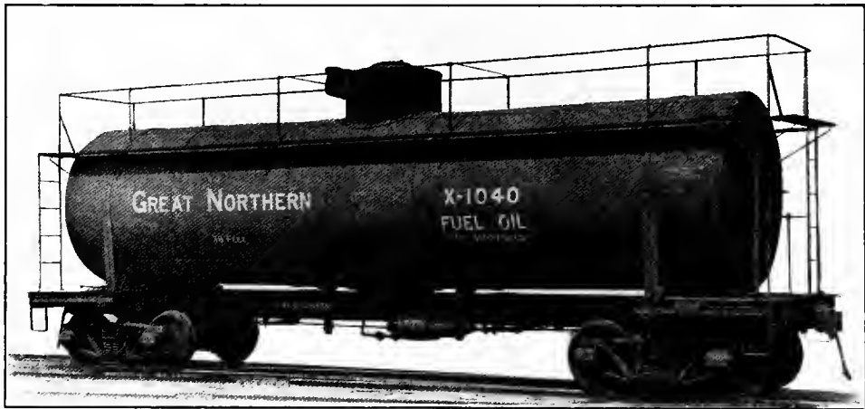
Fig. 83—Steel Frame Tank Car, Capacity, 12,000 U. S. Gallons or 100,000 lbs. Weight, 45,400 lbs. Builder, Pressed Steel Car Co.
