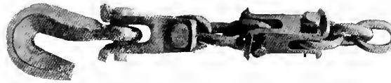
Fig. 2659—Buckley Wreck Chain Repair Link, Used on the Illinois Central for Temporary Repairs to Broken Chains.
