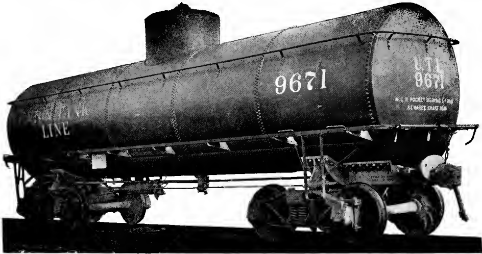
Fig. 88—Van Dyke Patent Tank Car, Capacity, 10,000 U. S. Gallons.
