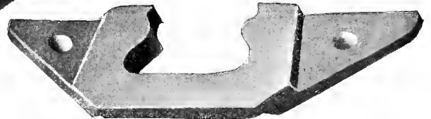
Fig. 1061—Side Plate of Carrier for Cardwell Rocker Side Bearing.
