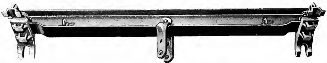
Fig. 1157—Acme Brake Beam for Short Wheel Base Freight Car Trucks. Simplex Railway Appliance Company.
