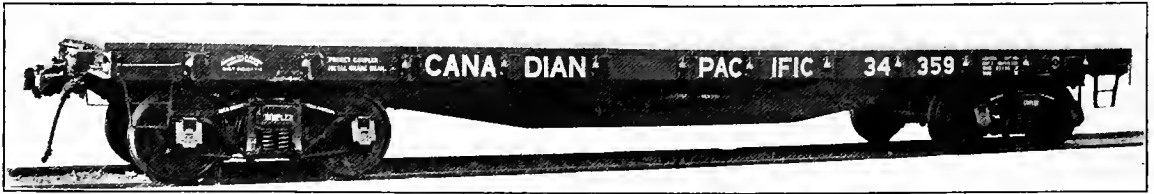
Fig. 68—Steel Frame 40-Ton Capacity Flat Car. Weight, 33,100 lbs.; Length of Platform, 41 ft. 6 in.; Width of Platform, 9 ft.; Height, Rail to Top of Platform, 4 ft. 2 \frac{3}{4} in. Builder, Canadian Car & Foundry Co.
