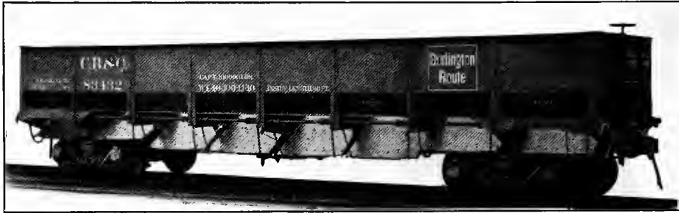
Fig. 49—All-Steel 50-Ton Capacity Drop-Bottom Gondola Car. Weight, 40,300 lbs.; Inside Length, 40 ft.; Inside Width, 9 ft. 6¾ in.; Inside Height, 4 ft. 2 in. Builder, Pressed Steel Car Co.
