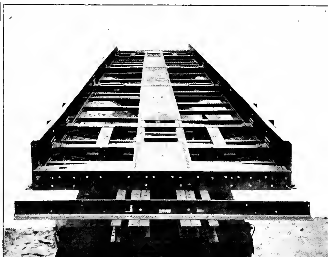
Fig. 464—Steel Underframe for Atlantic Coast Line Day Coach. Builder, Central Locomotive & Car Works.
