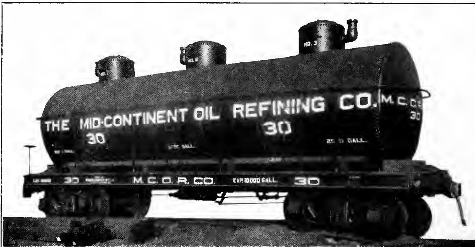
Fig. 84—Steel Frame Tank Car with Three Compartments. Capacity, 10,000 U. S. Gallons or 80,000 lbs. Builder, McGuire-Cummings Manufacturing Co.
