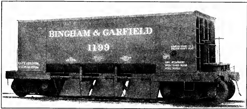
Fig. 31—All-Steel 60-Ton Capacity Ore Car. Weight, 42,300 lbs.; Inside Length, 23 ft. 10 \frac{3}{4} in.; Inside Width, 9 ft. 10 in.; Inside Height, 6 ft. 9 \frac{1}{2} in. Builder, Pressed Steel Car Co.
