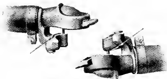
Fig. 1310—Hose Protecting Coupling.
