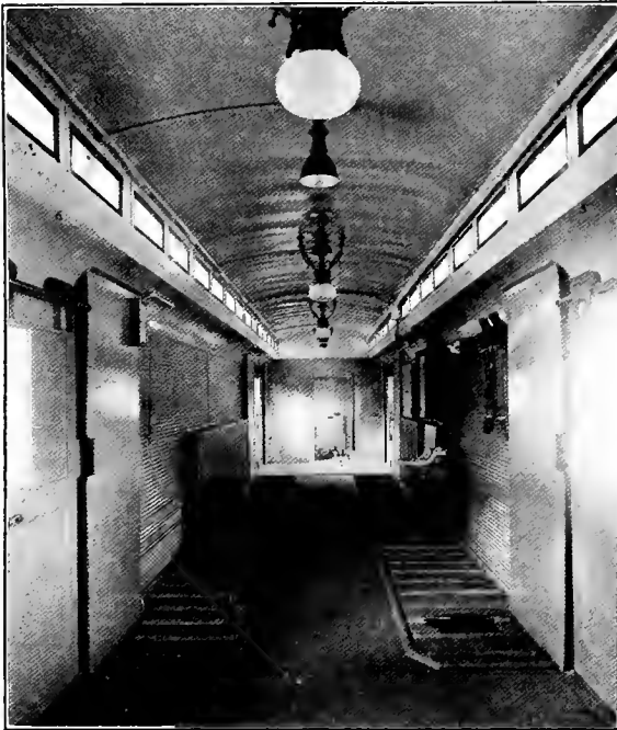
Fig. 127—Interior View of Steel Baggage Car Shown in Fig. 126.
