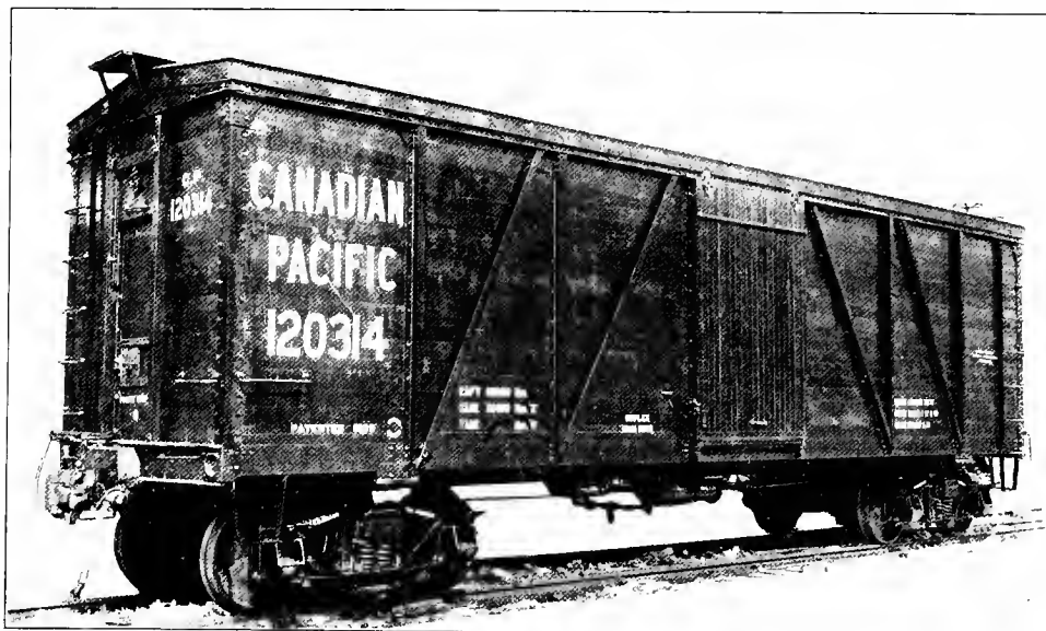
Fig. 6—Steel Frame 40-Ton Capacity Box Car, Fowler Patents. Weight, 36,400 lbs.; Inside Length, 36 ft.; Inside Width, 8 ft. 6 \frac{1}{2} in.; Inside Height, 8 ft. 0 \frac{1}{2} in. Builder, Canadian Car & Foundry Co. (See Figs. 267 and 268 for General Drawings)
