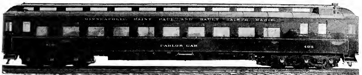
Fig. 175—Steel Vestibuled Parlor Car. Weight, 135,600 lbs.; Length Over Buffers, 80 ft. 4¾ in. Builder, The Barney & Smith Car Company.
