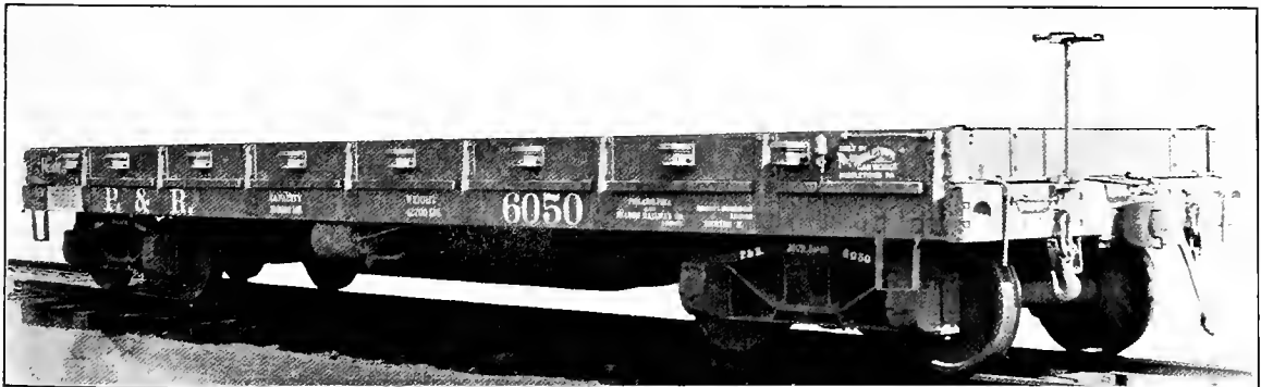
Fig. 55—Steel Underframe 50-Ton Capacity Low Side Solid Bottom Gondola Car. Weight, 42,700 lbs.; Inside Length, 36 ft. 4 in.; Inside Width, 8 ft. 9 in.; Inside Height, 1 ft. Capacity Level Full, Cubic Feet, 319. Builder, Middletown Car Co.
