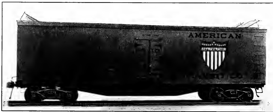
Fig. 107—Steel Underframe 30-Ton Capacity Refrigerator Car. Weight, 49,800 lbs.; Inside Length, 32 ft. 10 in.; Inside Width, 8 ft. 3 \frac{3}{8} in.; Inside Height, 7 ft. 6 in. Builder, American Car & Foundry Co.
