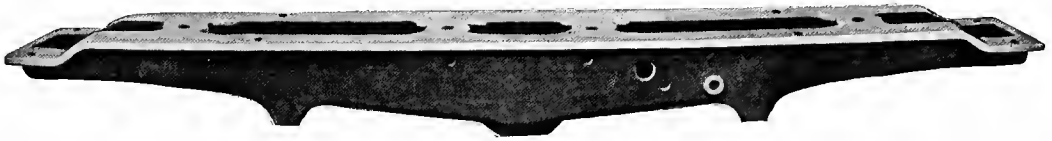
Fig. 515—Keystone Type Double Web Cast Steel Body Bolster. American Steel Foundries.
