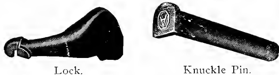
Fig. 628—Parts of Simplex Freight Coupler Simplex Railway Appliance Company.
