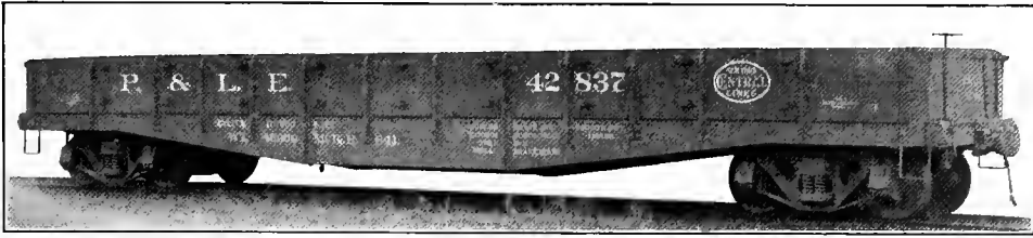
Fig. 52—Steel Frame 55-Ton Capacity Solid Bottom Gondola Car with Drop Ends. Weight, 46,000 lbs.; Inside Length, 46 ft.; Inside Width, 8 ft. 9 in.; Inside Height, 2 ft. 6¼ in.; Capacity Level Full, Cubic Feet, 1,015. Builder, Pressed Steel Car Co.
