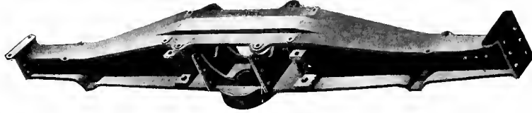
Fig. 516—Commonwealth Steel Company's Cast Steel Separable Body Bolster for Steel Freight Cars.
