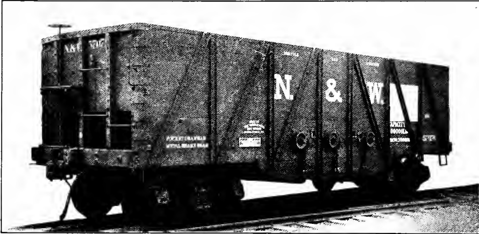
Fig. 23—Steel-Frame 50-Ton Capacity Hopper Car. Weight, 38,600 lbs.; Inside Length, 30 ft. 9 in.; Inside Width, 8 ft. 9½ in. Capacity Level Full Cubic Feet, 1,595. Builder, Middletown Car Co.
