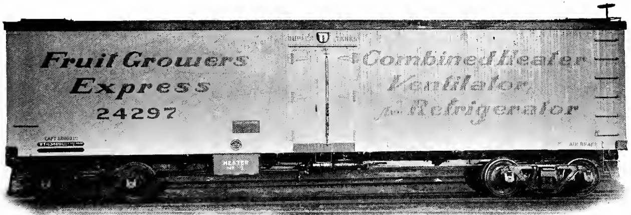
Fig. 118—Steel Underframe 30-Ton Capacity Combined Heater, Ventilator and Refrigerator Car. Weight, 43,400 lbs. This Car is Equipped with the Alcohol Heating & Lighting Co.'s Heater System.
