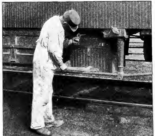
Fig. 2269—Generator Box Closed in Running Position. Dayton Manufacturing Company.
