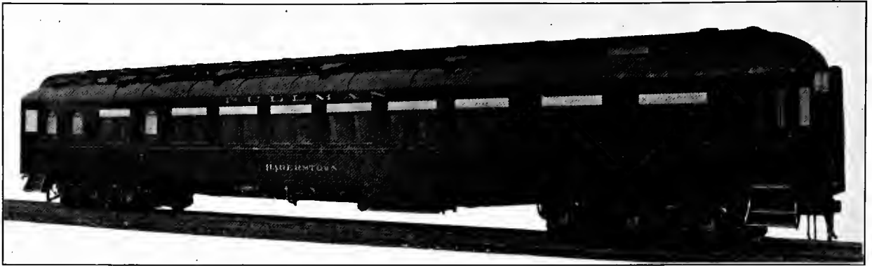
Fig. 176—Steel Vestibuled Sleeping Car. Weight, 150,000 lbs. Builder, The Pullman Company. (See Fig. 181 for Interior View and Figs. 411-414, 416-418 and 420 for General Drawings.)
