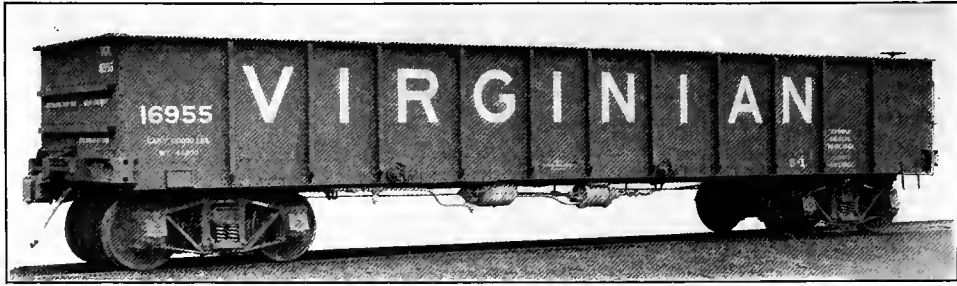
Fig. 48—All-Steel 50-Ton Capacity Drop-Bottom Gondola Car. Weight, 43,200 lbs.; Inside Length, 40 ft.; Inside Width, 9 ft. 4 in.; Inside Height, 4 ft. 6 in. Builder, Pressed Steel Car Co.
