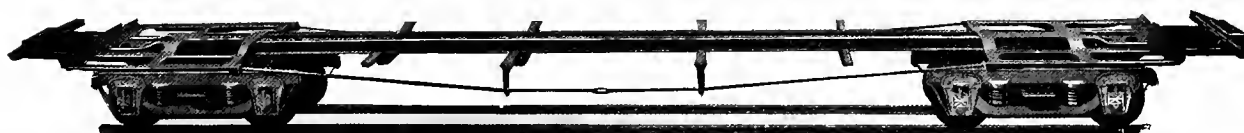
Fig. 456—Commonwealth Steel Company's Combined Steel and Wood Underframe for Passenger Train Cars, Using Cast Steel Combined Platform and Double Body Bolsters, Steel Cross Ties and Needle Beams.
