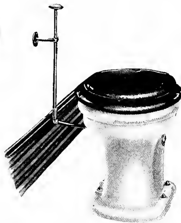
Fig. 1645—Americo Closet with Operating Lever on Side Wall. The Watrous Company.
