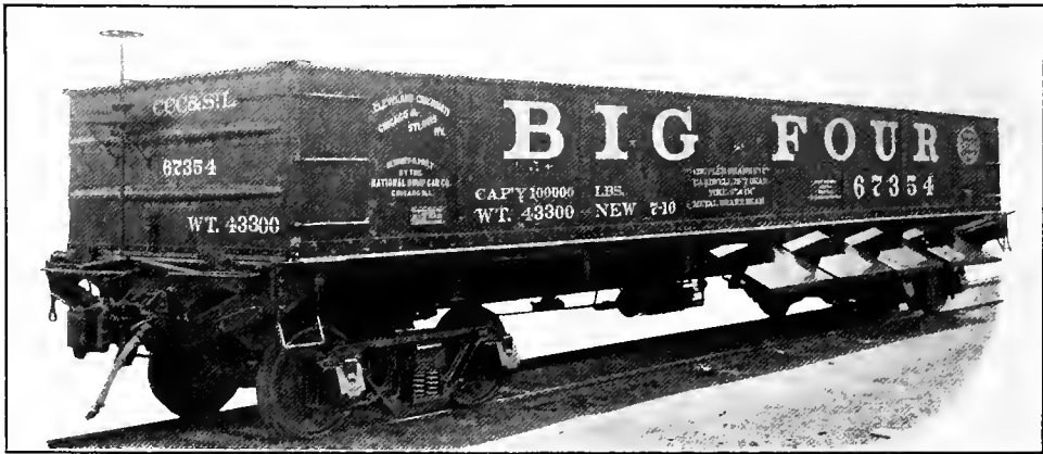
Fig. 41—All-Steel 50-Ton Capacity Drop-Bottom Gondola Car. Weight, 43,300 lbs.; Inside Length, 40 ft.; Inside Width, 9 ft. 6 in.; Inside Height, 4 ft. 3 in. Builder, National Dump Car Co.
