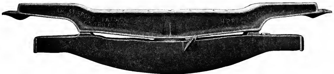
Fig. 1067—Cast Steel Truck and Body Bolsters for Freight Cars. American Steel Foundries.
