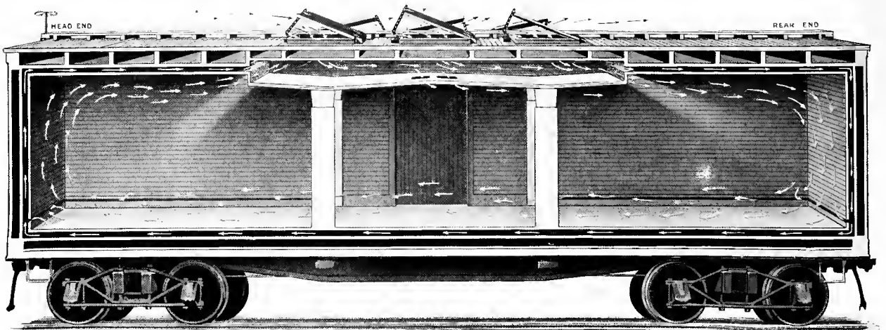
Fig. 855—Air Circulation in Moore Patent Car when Arranged for Ventilation. Moore Patent Car Company. See also Figs. 109 and 114.
