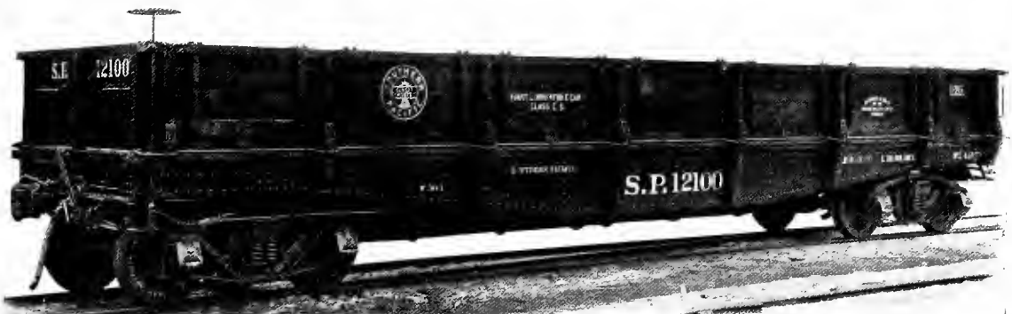
Fig. 40—Steel Underframe 50-Ton Capacity Hart Convertible Car. Weight, 41,800 lbs.; Inside Length (as Gondola), 40 ft.; Inside Width, 8 ft. 9 in.; Inside Height, 3 ft. 6 in. Builder, Rodger Ballast Car Co.
