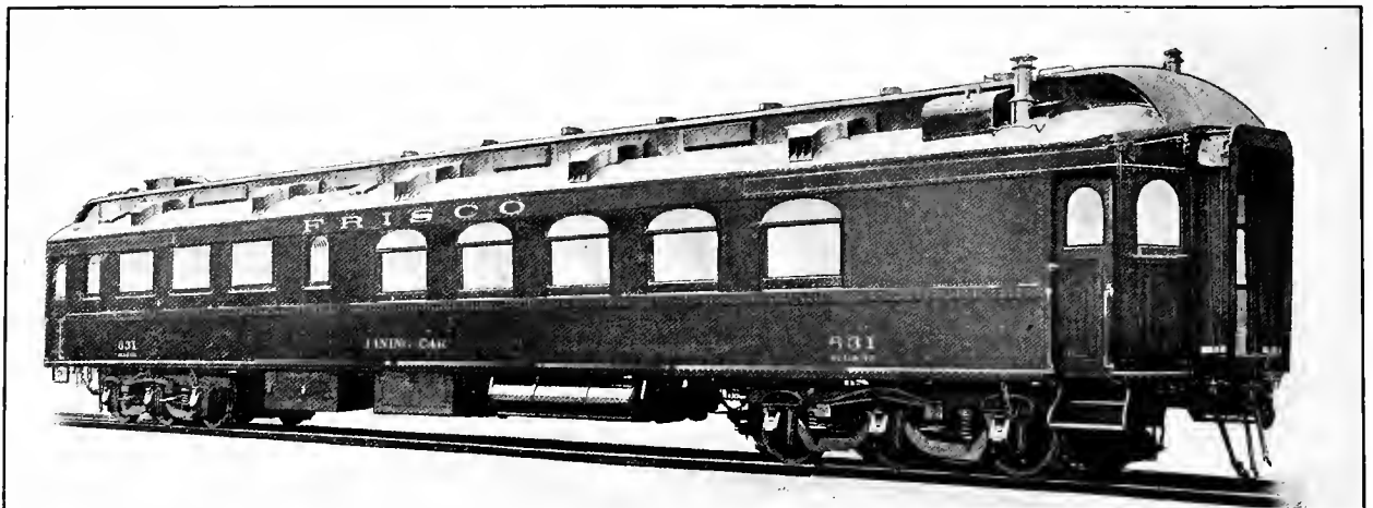
Fig. 161—Steel Vestibuled Dining Car. Builder, American Car & Foundry Co. (See Figs. 159, 160 and 163 for Interior Views.)
