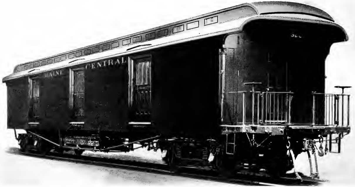
Fig. 100—Wooden Express Car for the Transportation of Horses. Builder, The Wason Manufacturing Co.
