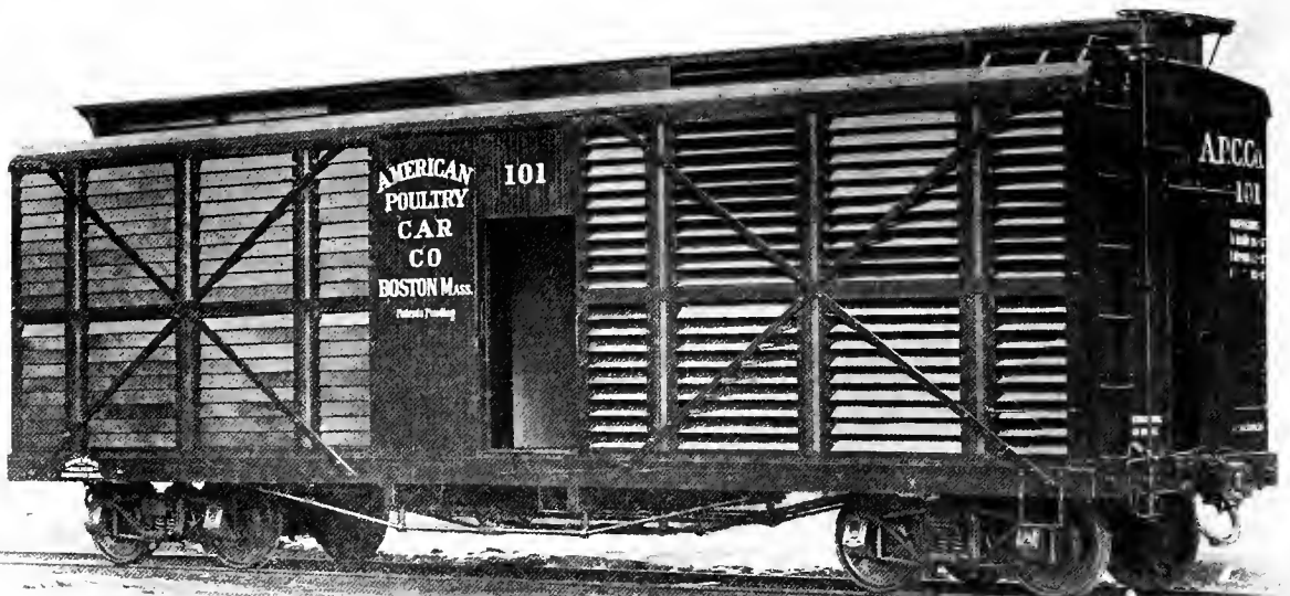
Fig. 96—Wooden Poultry Car with Clere-story. Builder, Wason Manufacturing Co.
