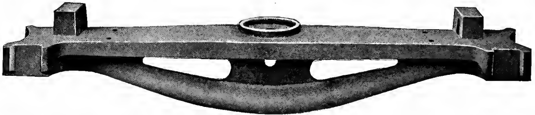
Fig. 1069—T-Shape Cast Steel Truck Bolster for Freight Cars. American Steel Foundries.
