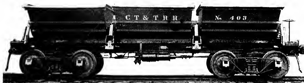
Fig. 67—All-Steel 12 Cubic Yards Capacity Two-Way Triple Body Side Dump Car. Builder, Arthur Kopple Co.
