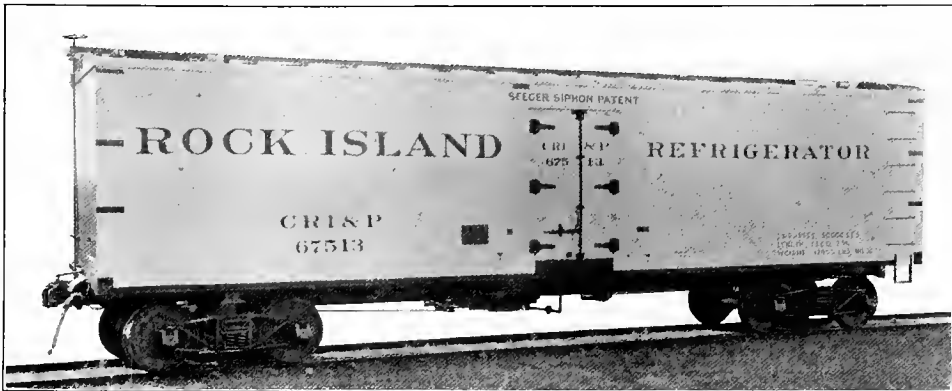
Fig. 106—Steel Underframe 30-Ton Capacity Refrigerator Car. Weight, 47,400 lbs.; Inside Length, 33 ft. 2 in.; Inside Width, 8 ft. 2 in.; Inside Height, 7 ft. 6 in. Builder, Milwaukee Refrigerator Transit & Car Co.
