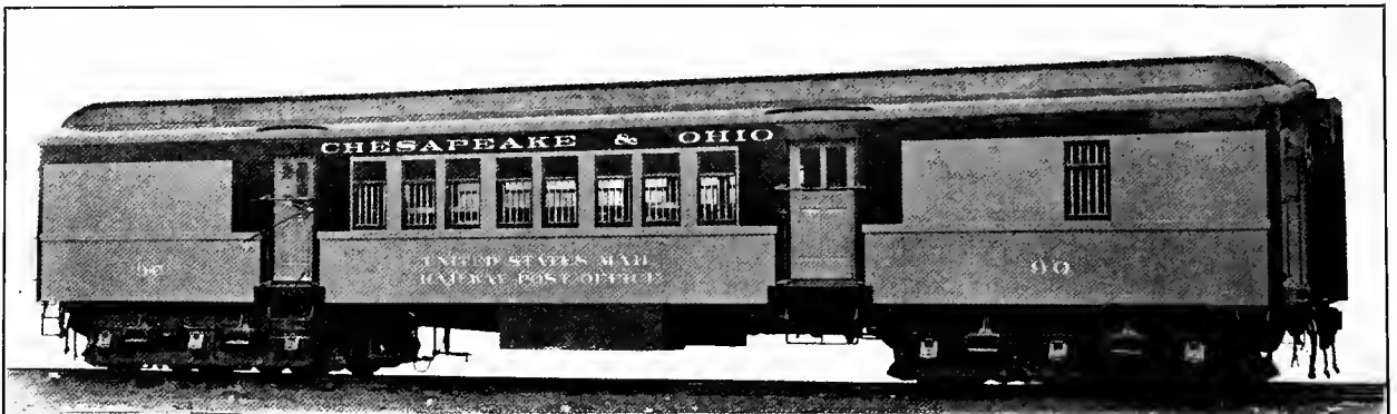
Fig. 137—Steel Postal Car. Weight, 113,200 lbs. Builder, Pressed Steel Car Co.
