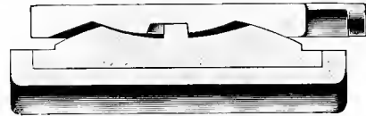
Fig. 1002—Section Through A. B. C. Journal Bearing and Wedge. A. B. C. Bearing Corporation.
