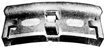
Reinforcing Steel Back and Steel Lug for Full, Open and Center Flange Brake Shoes.
