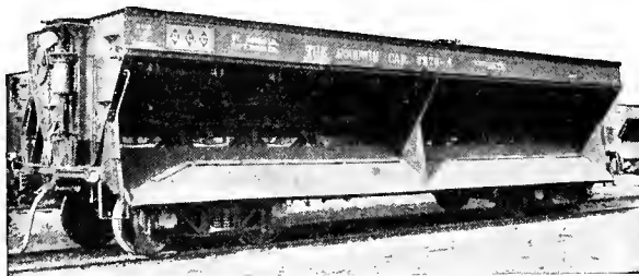
THE GOODWIN STANDARD CLASS "G" DUMP AND BALLASTING CAR AIR DUMPING AND AIR REPLACING
