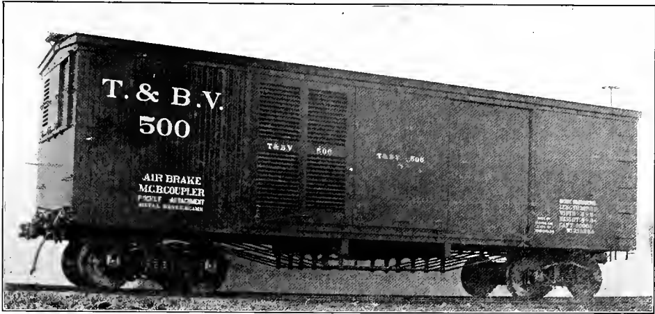
Fig. 116—Wooden 30-Ton Capacity Ventilating Car for Fruit Traffic. Weight, 33,800 lbs.; Inside Length, 36 ft. Builder, Georgia Car & Manufacturing Co.
