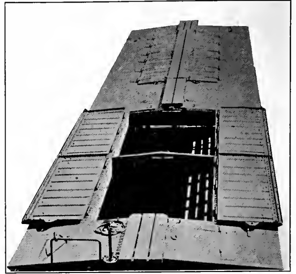
Fig. 863—Roof of General Service Car Shown in Fig. 92. National Dump Car Company.
