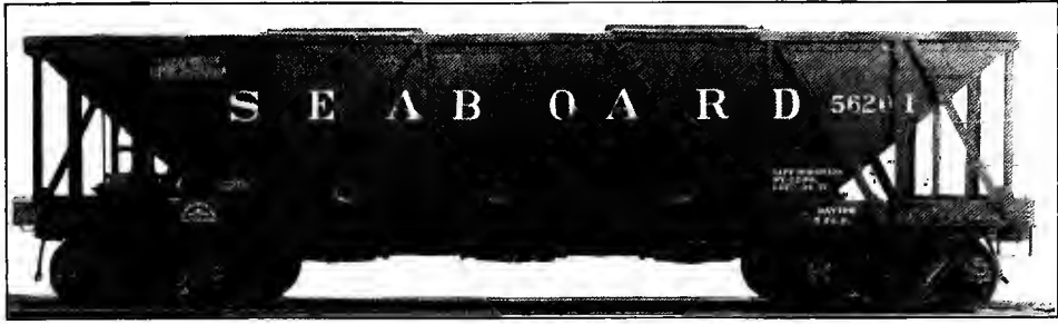
Fig. 19—All-Steel 50-Ton Capacity Hopper Car for Phosphate Traffic. Weight, 42,000 lbs.; Inside Length, 34 ft.; Inside Width, 9 ft. 1 \frac{3}{8} in.; Length Over End Sills, 37 ft. 2 in.; Height, Rail to Top of Body, 9 ft. 8 \frac{3}{4} in.; Extreme Height, 11 ft. 1 \frac{1}{4} in. Capacity Level Full, Cubic Feet, 1,615. Builder, The Barney & Smith Car Co.
