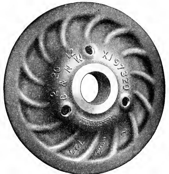
Fig. 1153—M. C. B. Standard Cast Iron Wheel for 50-Ton Capacity Freight Cars. Weight, 725 lbs. Association of Manufacturers of Chilled Car Wheels.
