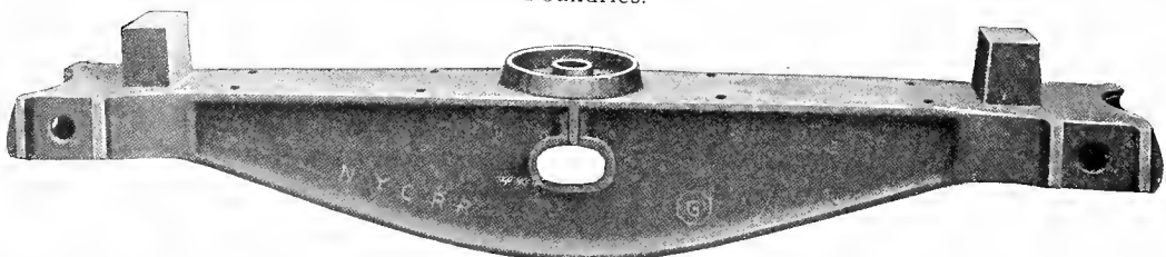
Fig. 1072—I-Shape Cast Steel Truck Bolster for 30 and 40-Ton Capacity Freight Cars. American Steel Foundries.
