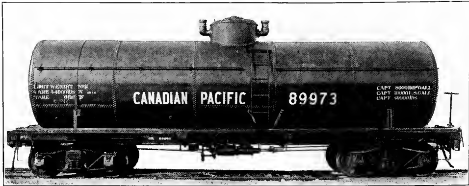
Fig. 82—Steel Frame Tank Car, Capacity, 8,000 Imperial Gallons or 40 Tons. Weight, 44,900 lbs.; Length of Tank, 33 ft. 6 in.; Extreme Height from Rail, 13 ft. 5 in. Builder, Canadian Car & Foundry Co.
