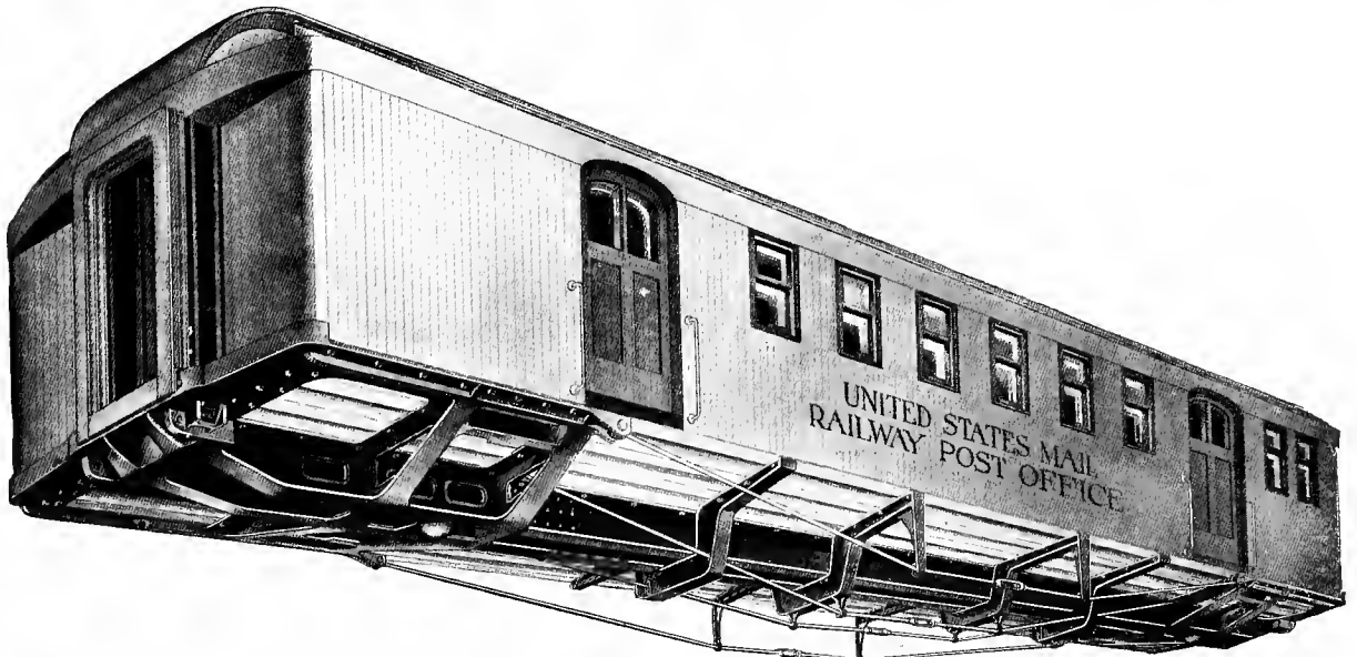
Fig. 446—Commonwealth Steel Company's Steel Underframe for Strengthening Old Postal Cars.
