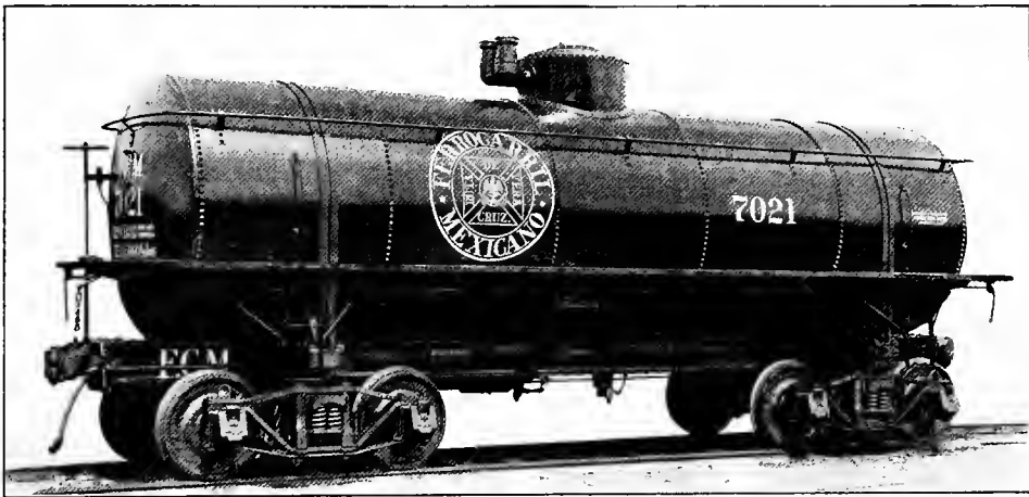
Fig. 86—Steel Frame Tank Car, Capacity, 8,000 U. S. Gallons. Builder, Pressed Steel Car Co.
