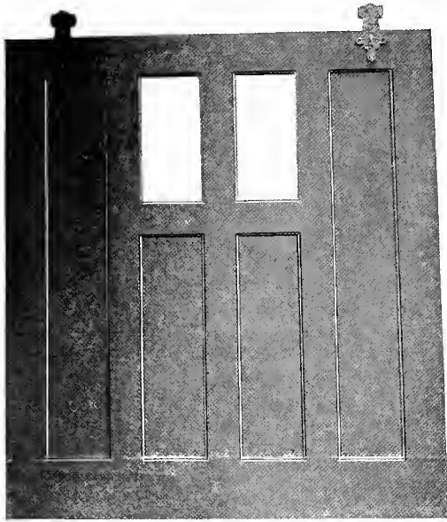
Fig. 818—Hollow Steel Baggage Car Door. Grinden Art Metal Company.
