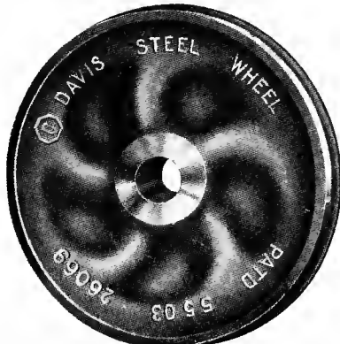
Fig. 1141—Davis Cast Steel Wheel. Weight of 33 in., 600 lbs.; 36 in., 675 lbs. American Steel
