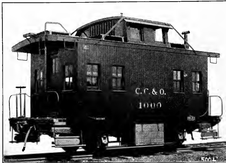
Fig. 119—Steel Underframe Four-Wheel Caboose. Builder, Central Locomotive & Car Works.
