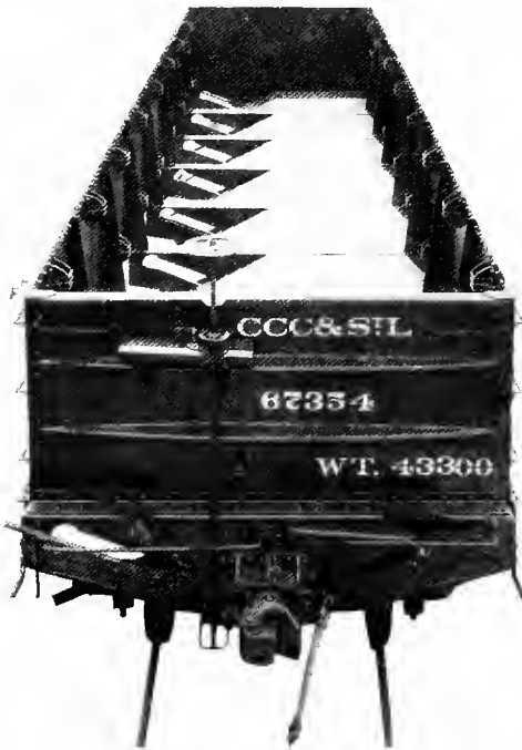
Fig. 42—Drop-Bottom Gondola Car with Doors Open on One Side. Fig. 43—Drop-Bottom Gondola Car with all Doors Open. Builder, National Dump Car Co.
