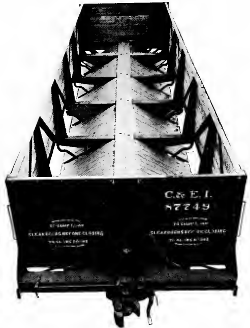
Fig. 42—Drop-Bottom Gondola Car with Doors Open on One Side. Fig. 43—Drop-Bottom Gondola Car with all Doors Open. Builder, National Dump Car Co.
