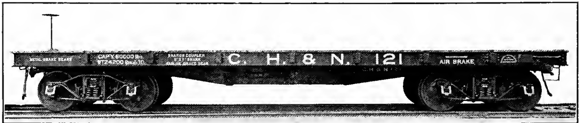
Fig. 69—Steel Frame 30-Ton Capacity Flat Car. Weight, 24,200 lbs. Builder, The Barney & Smith Car Co.
