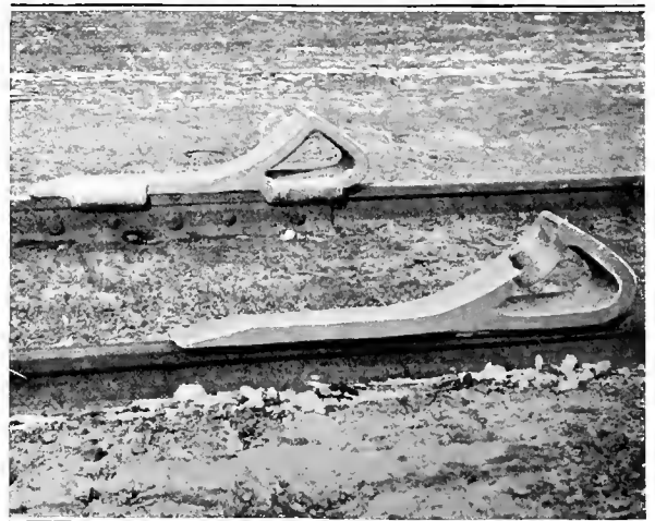
Fig. 2649—R. A. Skid Shoe for Sliding Damaged Wheels.
