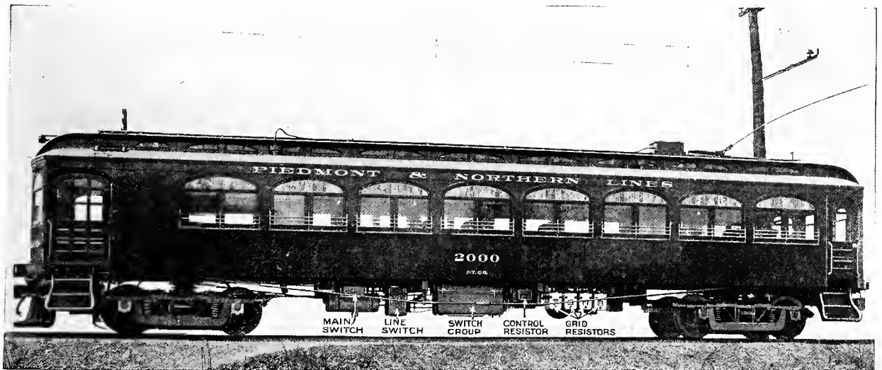
Fig. 2536—Motor Car Equipped with 1,500 Volt, Direct Current Apparatus.
