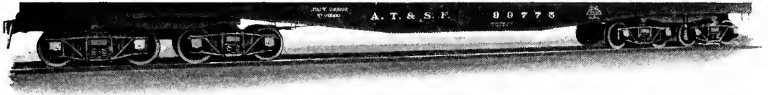
Fig. 72—Steel Frame 100-Ton Capacity Four-Truck Flat Car. Weight, 90,000 lbs.; Length of Platform, 70 ft. 7 in.; Width of Platform, 8 ft. 6 in. Builder, McGuire-Cummings Manufacturing Co.
