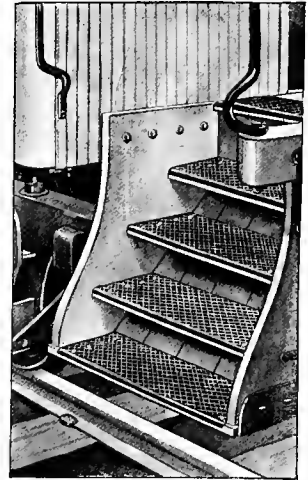
Fig. 610 — Feralun Safety Tread Applied to Car Steps. American Abrasive Metals Company.
