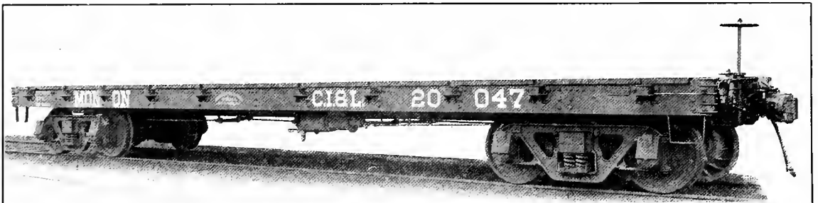
Fig. 74—Steel Frame 40-Ton Capacity Flat Car. Weight, 30,700 lbs.; Length of Platform, 40 ft.; Width of Platform, 8 ft. 6 in. Builder, The Haskell & Barker Car Co.
