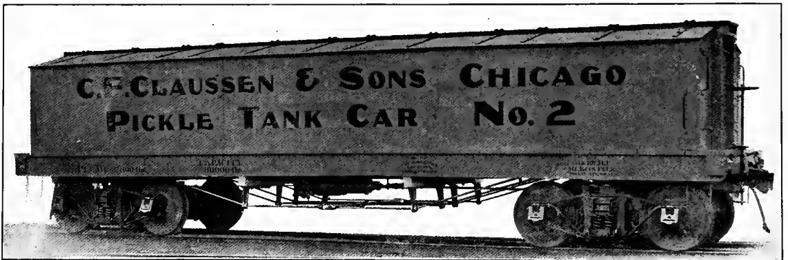
Fig. 89—Three Compartment 30-Ton Capacity Tank Car for Pickle Transportation. Weight, 37,300 lbs. Builder, Middletown Car Co.
