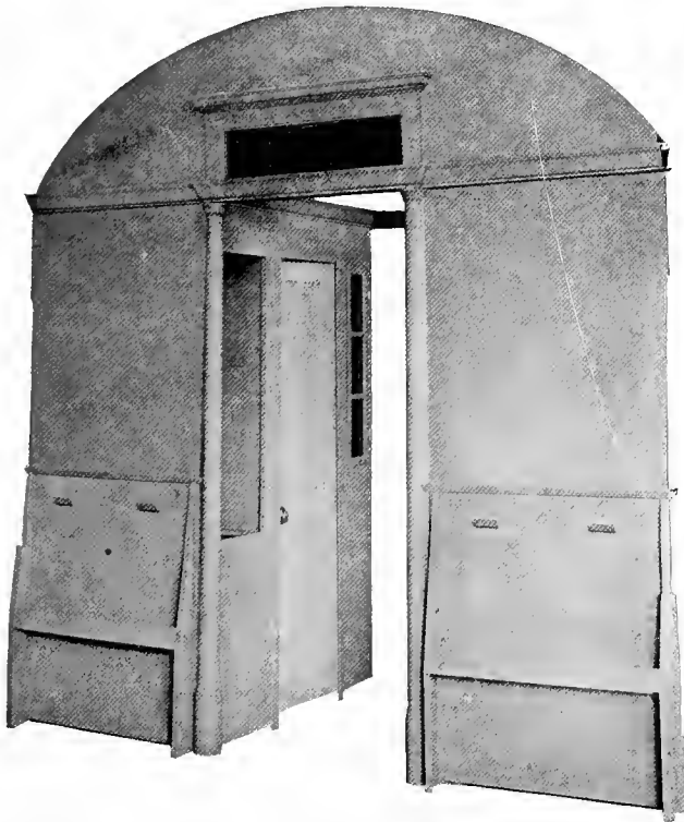
Fig. 1451—Steel Bulkhead and Saloon for Harriman Lines Arched Roof Coach. Hale & Kilburn Company.
