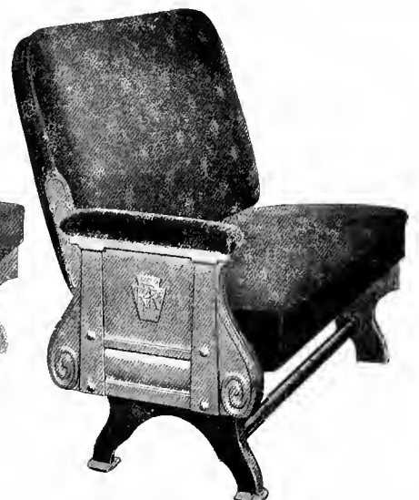
Fig. 1519—Steel Walkover Seat with Frieze Plush Upholstery, for Pennsylvania Railroad Steel Coaches.
