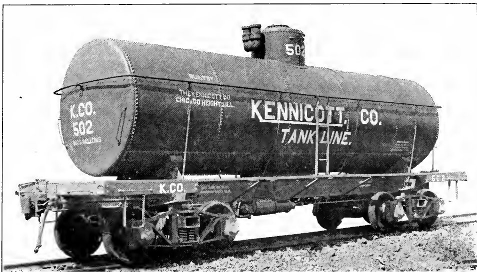
Fig. 87—Steel Frame Tank Car, Capacity, 8,000 U. S. Gallons or 80,000 lbs.; Weight, 35,300 lbs. Builder, The Kennicott Co.
