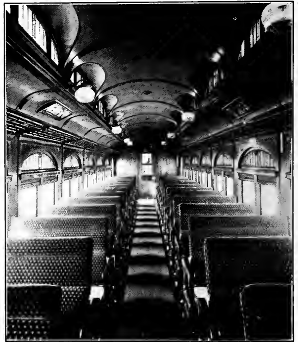
Fig. 144—Interior View of New York Central Lines Day Coach. The Interior Finish is Wood. Builder, The Barney & Smith Car Co.
