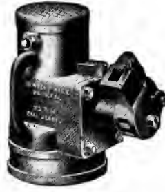
Fig. 2637—Ball Bearing Journal Jack with Wheel Holding Device.
