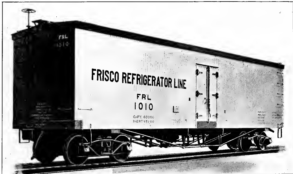
Fig. 111—Wooden 30-Ton Capacity Refrigerator Car with Steel Center Sills. Weight, 45,100 lbs.; Inside Length, 33 ft.; Inside Width, 8 ft. 4 in.; Inside Height, 7 ft. 6 in. Builder, American Car & Foundry Co.
