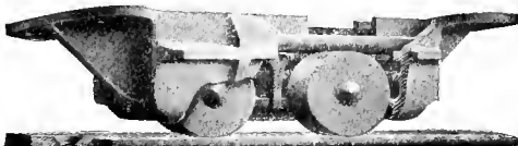
Fig. 1036—Double Roller Side Bearing. Edwin S. Woods & Company.
