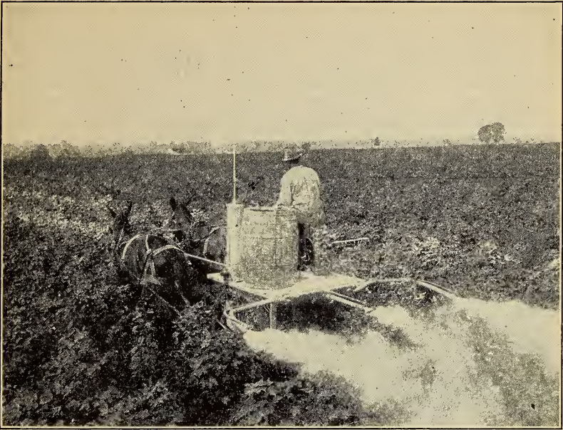
FIG. 8.—The cart dusting machine has two wheels that straddle a row of cotton, and it is drawn by two mules or horses
