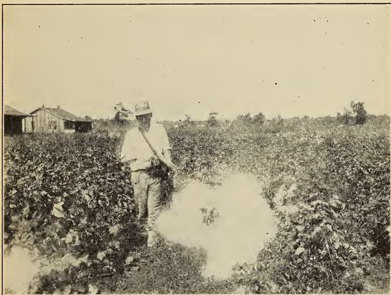
FIG. 6.—The hand dust gun is the smallest kind of machine for dusting cotton plants with calcium arsenate to kill boll weevils. The man who uses it turns a crank which causes a fan to blow the poison dust out of the long nozzle sticking out of the front.
