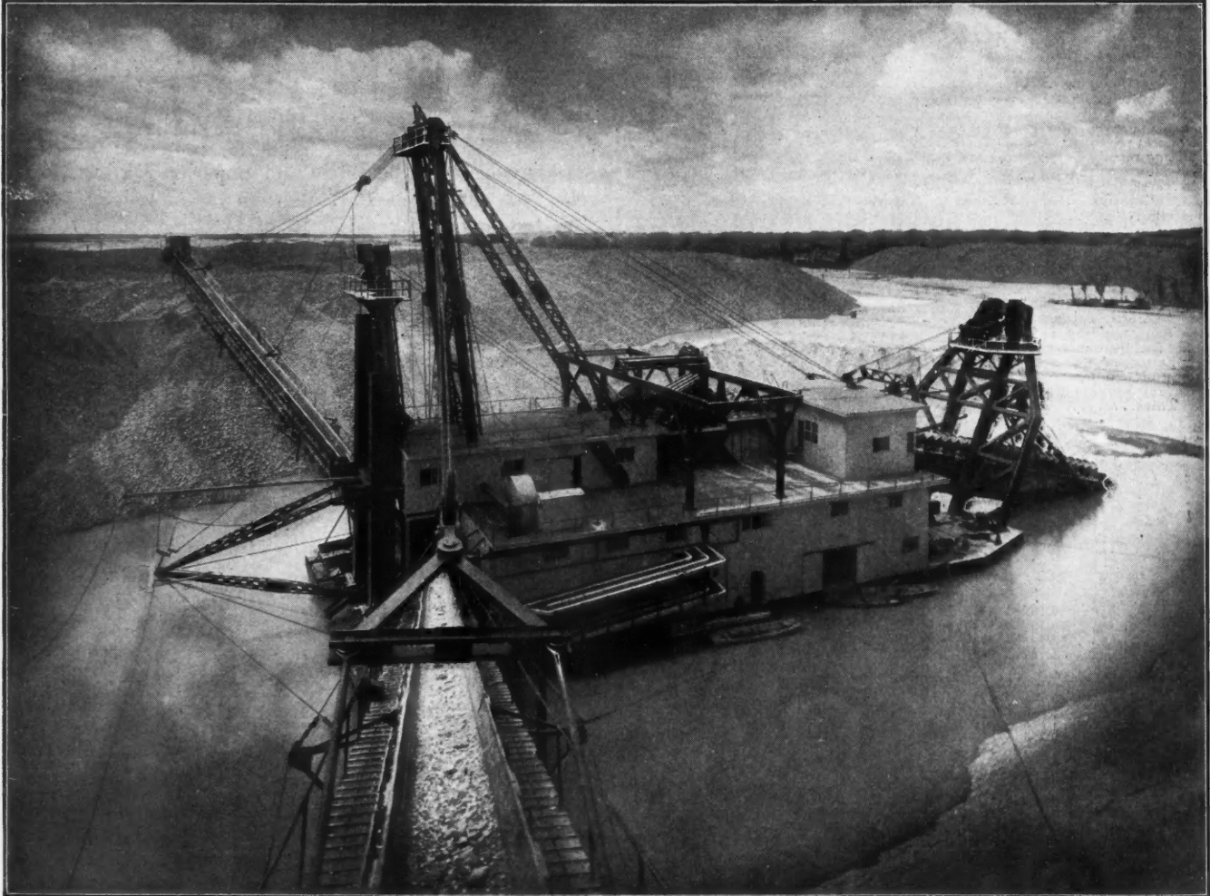
YUBA NO. 16 DOUBLE-STACKER GOLD DREDGE WHICH STARTED DIGGING AT HAMMONTON, CALIF., IN APRIL
